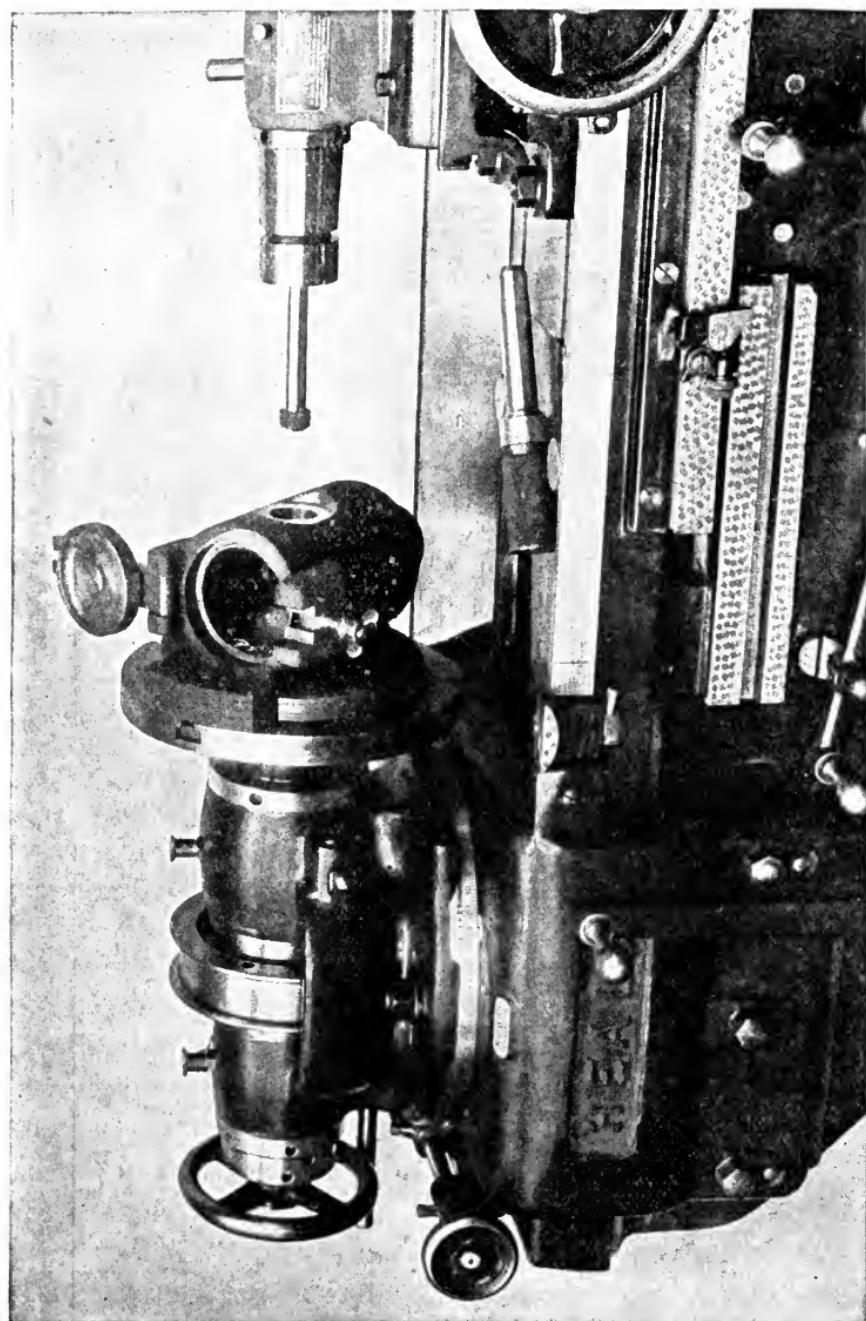
Fig. 336. Set-Up for Grinding Wrist-Pin Bearing; Grinding Time 3 Minutes per Piston
