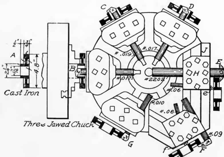
Fig. 310. Arrangement for Machining Spur-Gear Blank
