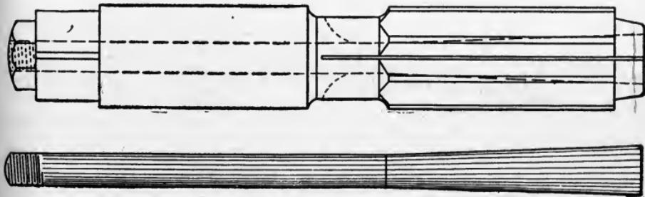
Fig. 77. Expanding Reamer and Arbor
