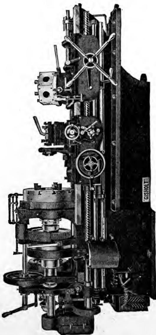
Fig. 297. "I" 24-Inch Turret Lathe with Motor Drive
