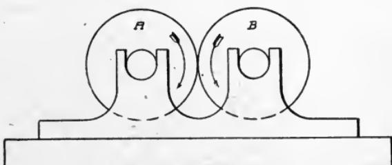
Fig. 258. Two Cylinders in Contact
