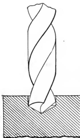
Fig. 70. Drill with Lips of Unequal Angles
