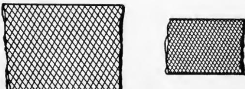
Fig. 50. Diagram Showing Coarseness of Files
