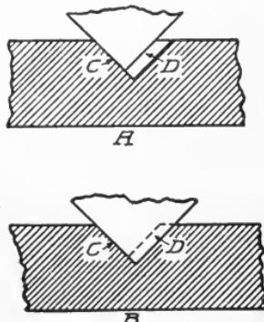
Fig. 180. Action of Groove in Making Drill Hole Concentric
