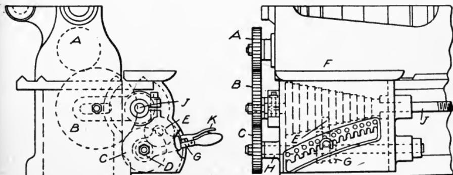
Fig. 99. End and Front Elevation of Rapid Change-Gear Device
