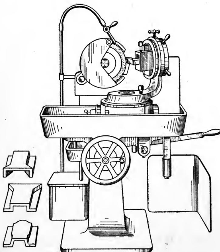
Fig. 132. Tool-Grinding Machine
