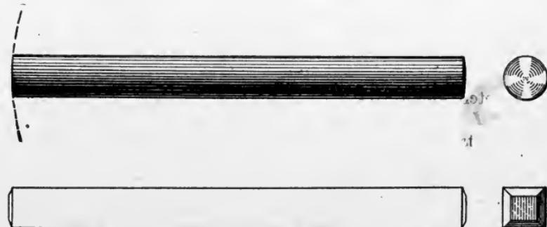
Fig. 33. End Measuring Rods
