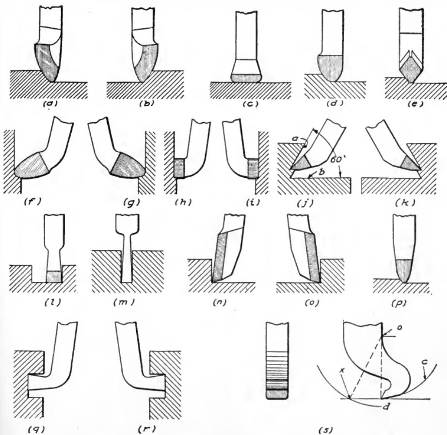
Fig. 372. Planer Tools of Different Form and Work to Which They Are Adapted
