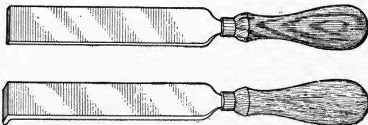
Fig. 58. Straight and Bent Hand Scrapers
