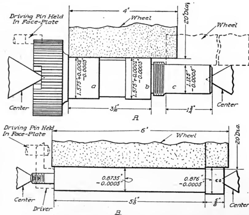
Fig. 333. Diagram of Set-Ups Shown in Figs. 331 and 332
