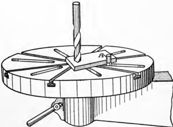
Fig. 182. Use of Table Stud for Drilling
