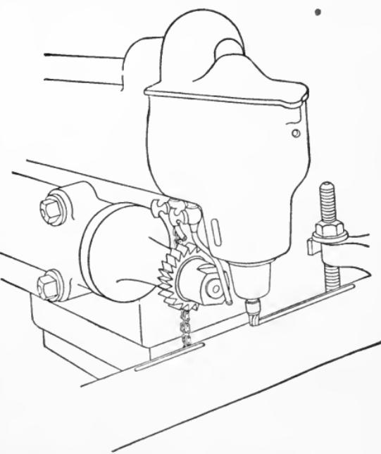
Fig. 235. Splining Arrangement with End Mill in Vertical Head
