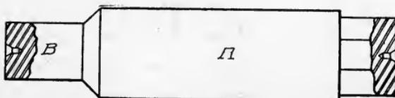
Fig. 111. Stuffing-Box Gland Requiring Special Mandrel
