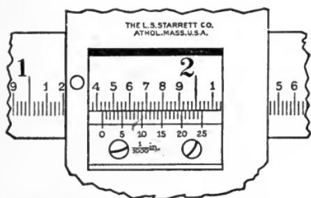
Fig. 25. Enlarged View of Vernier
