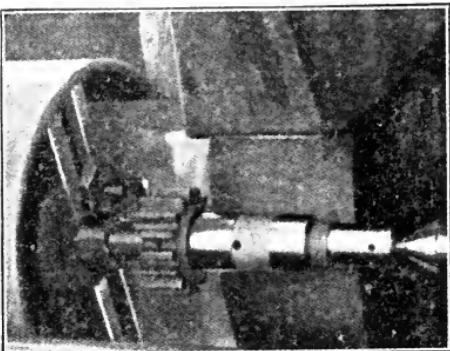
Figs 331 and 332. Set-Up for Grinding
