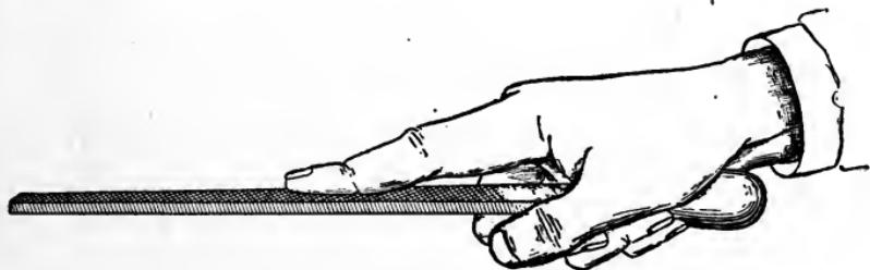
Fig. 54. Position for Single Hand Filing
