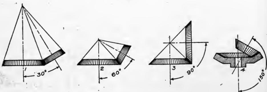
Fig. 270. Bevel Gears at Various Angles
