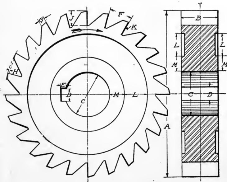
Fig. 200. Details of Ordinary Milling Cutter
