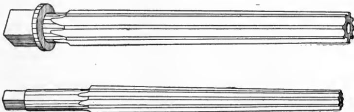
Fig. 79. Types of Taper Reamers
