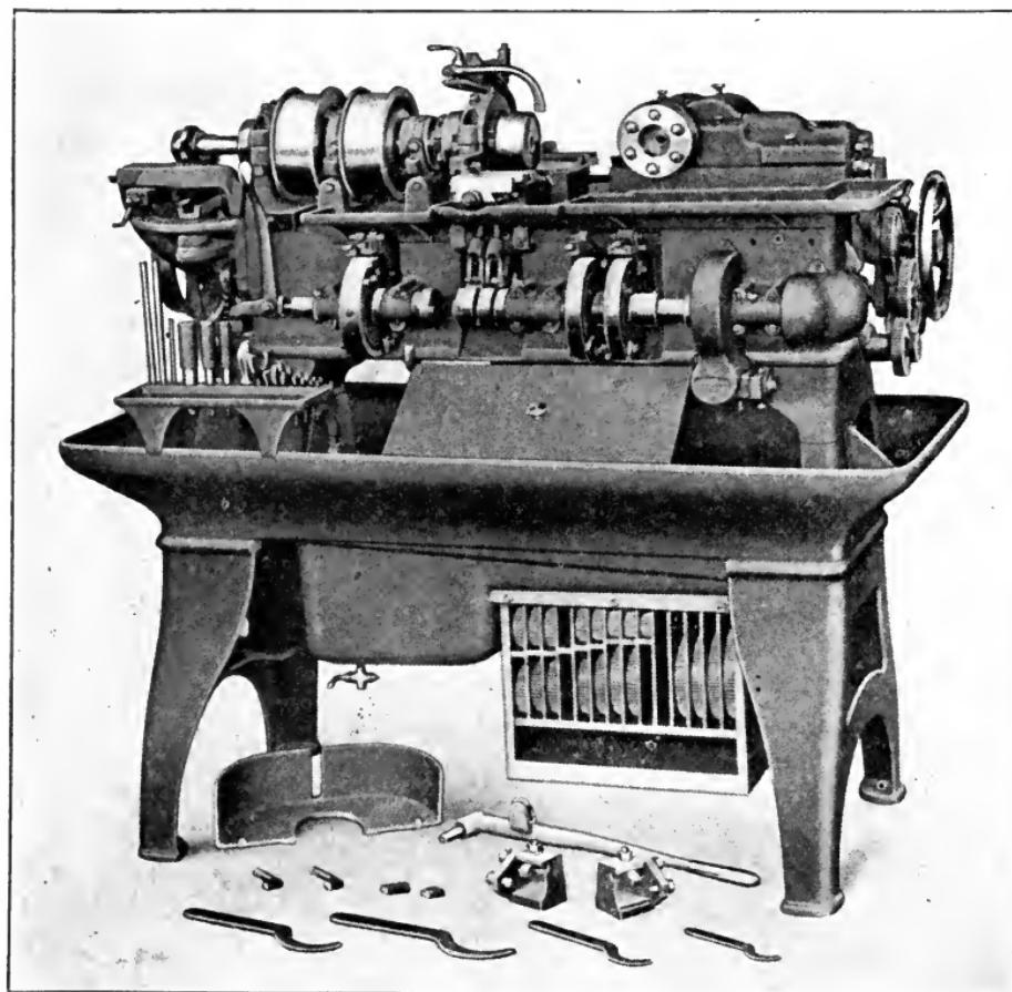
Fig. 321. Number 2 Automatic Screw Machine
