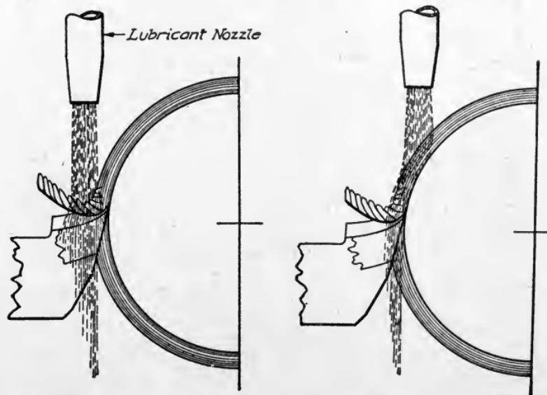
Fig. 373. Right and Wrong Method of Feeding Lubricant to Cutting Tool
