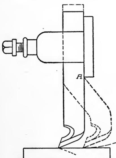
Fig. 186. Incorrect and Correct Setting for Planer Tool
