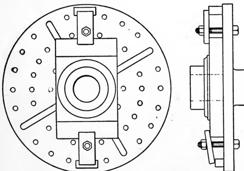
Fig. 135. Work Clamped to Faceplate
