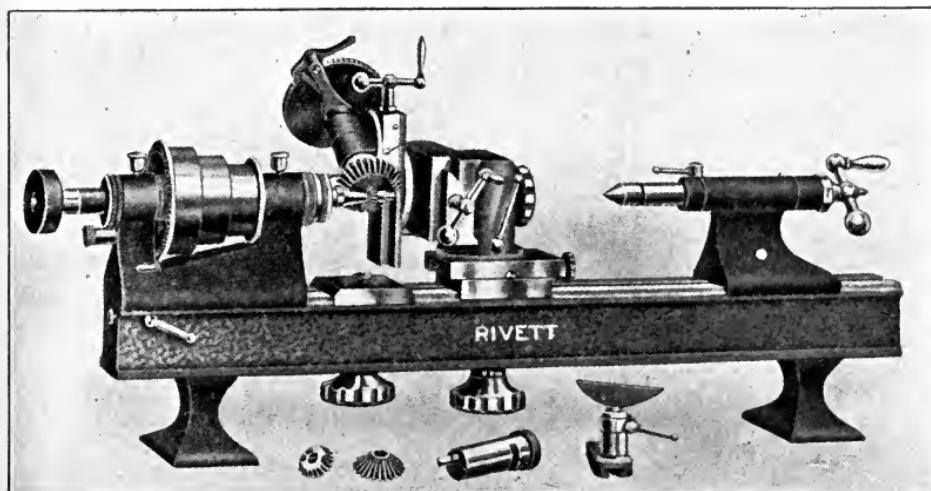
Fig. 222. Rivett Lathe with Milling Attachment
