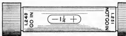
Fig. 39. Limit Gage for Holes
