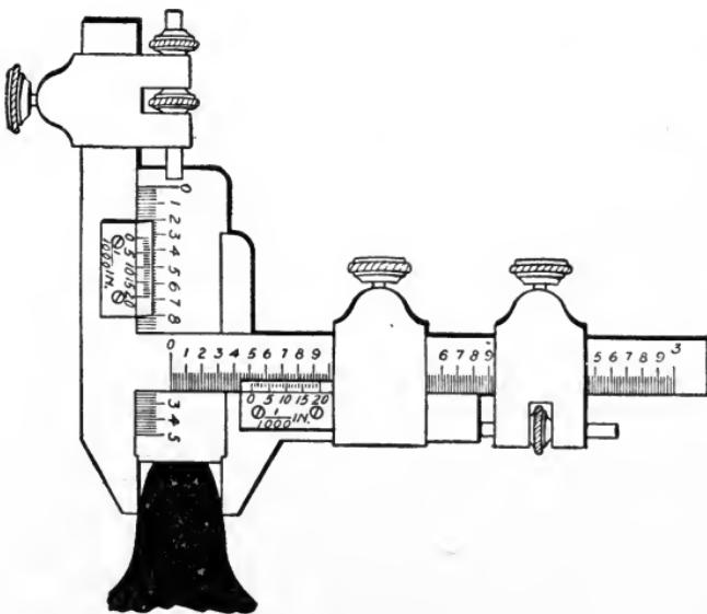
Fig. 280. Gear-Tooth Caliper in Use
