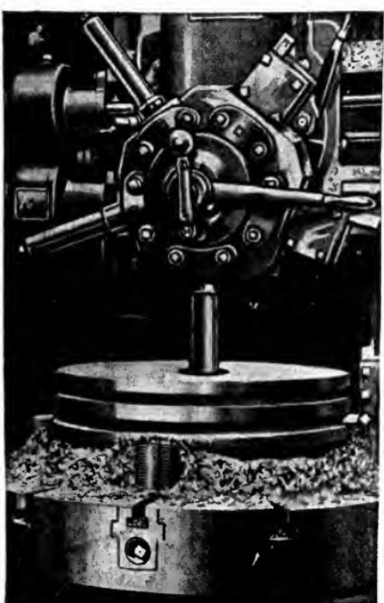
cutting tools. Both long and short turning can be done in this machine. The turret provides for six tools.
