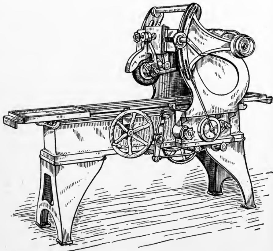
Fig. 248. Surface-Grinding Machine
