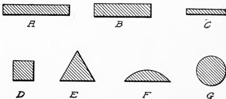
Fig. 49. Cross-Section of Files
