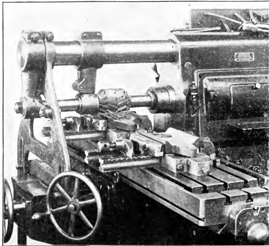
Fig. 341. Horizontal Milling Machine with Work in Process
