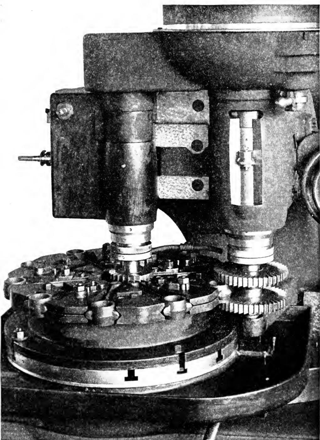
**VIEW OF BECKER CONTINUOUS MILLER MILLING CONNECTING-ROD FIXTURE**
