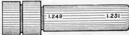
Fig. 40. Limit Gage for Holes with Limits in Series
