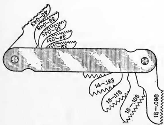
Fig. 163. Screw Pitch Gage
