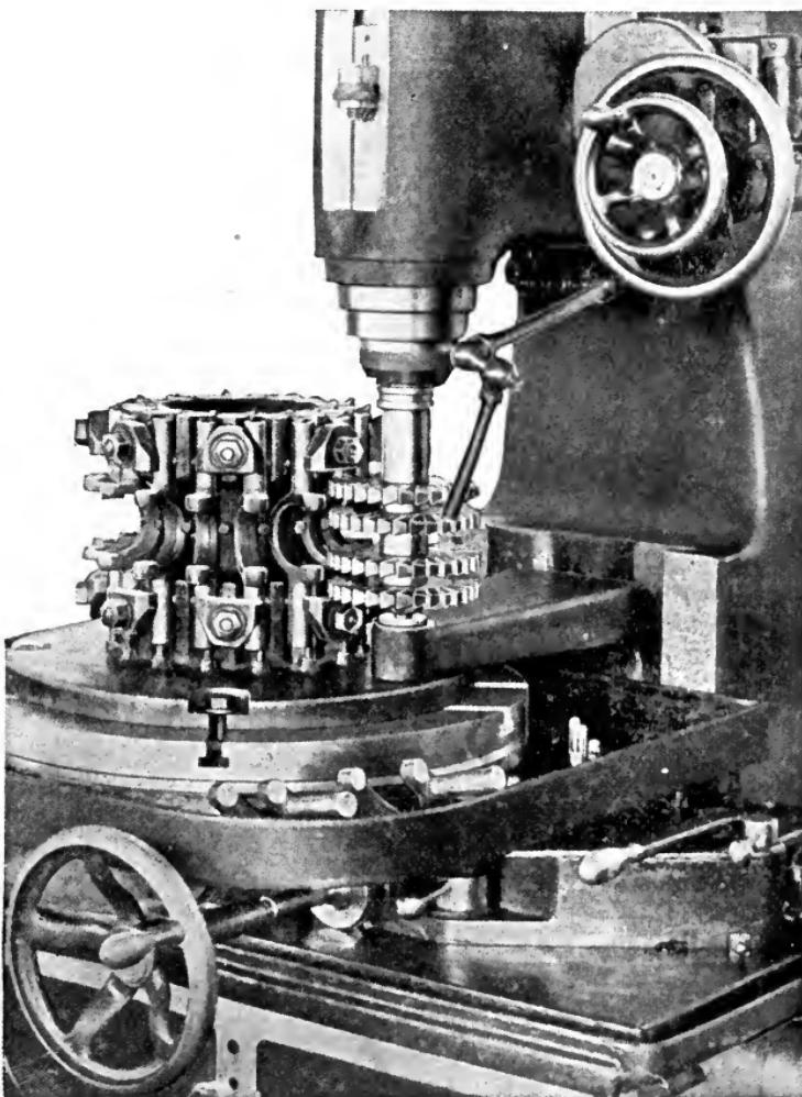
Fig. 342. Vertical Milling Machine in Action. Work-Holding Fixture Rotates at Rate of 10 Inches per Minute; Production 195 Yokes per Hour
