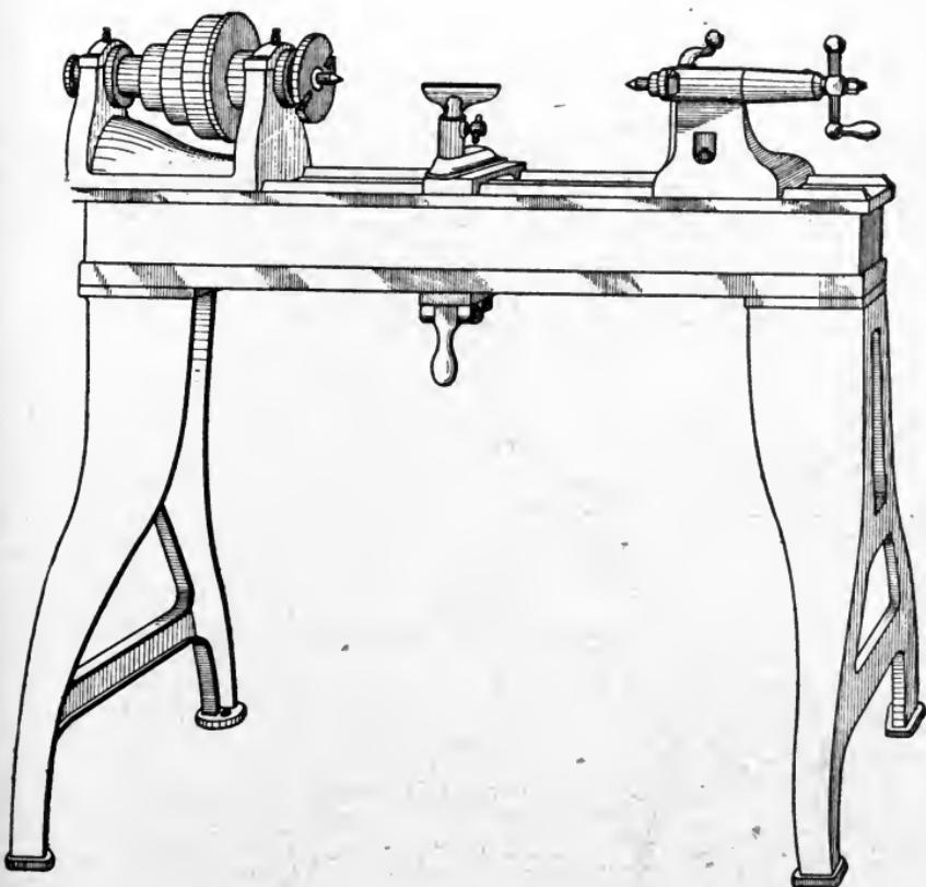
Fig. 87. Typical Speed Lathe for Hand Turning
