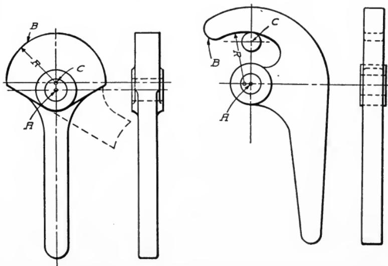
Fig. 383. Diagrams Showing Cams or Eccentrics Used for Clamping
