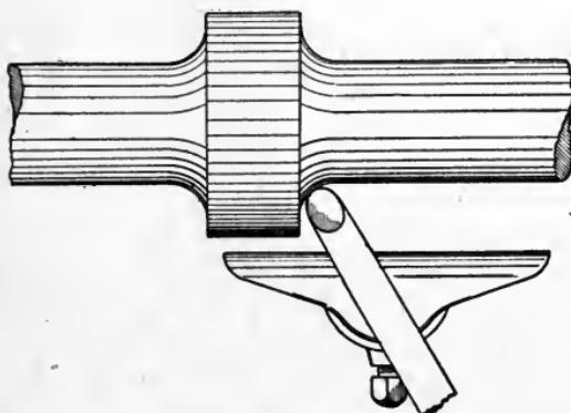
Fig. 93. Hand-Turning a Fillet
