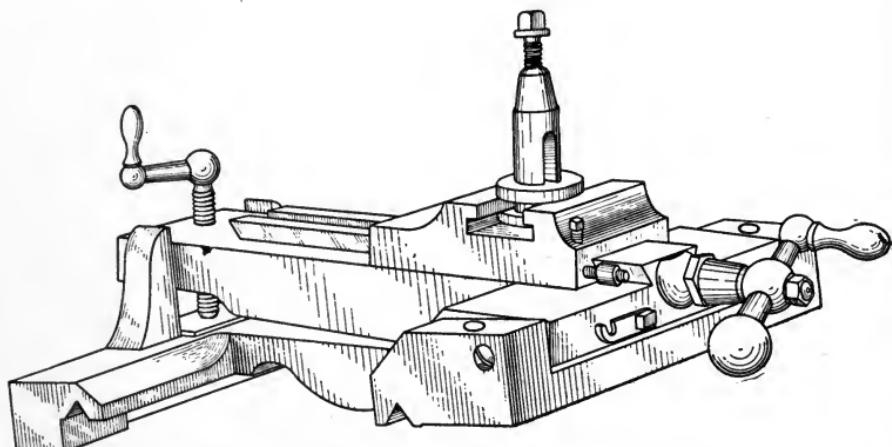
Fig. 122. Tool-Post with Rise-and-Fall Rest
