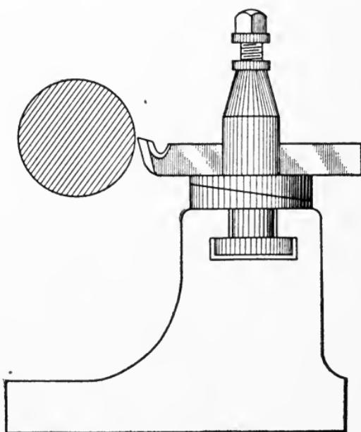
Fig. 120. Bevel Ring Tool-Post
