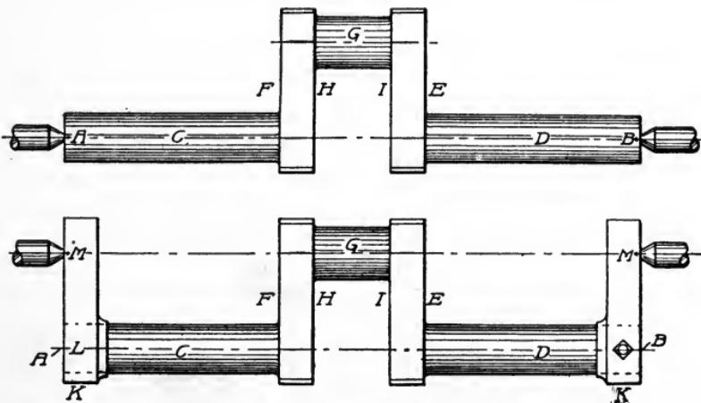
Fig. 148. Machining Crank Shaft
