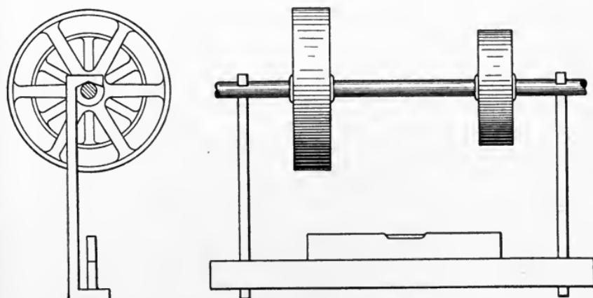
Fig. 257. Method of Using Level for Lining Shafting
