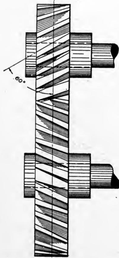
Fig. 275. Simple Form of Spiral Gears
