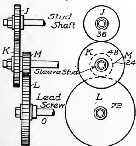
Fig. 98. Compounding Gears
