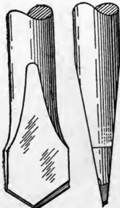
Fig. 172. Flat Drill of Simplest Type
