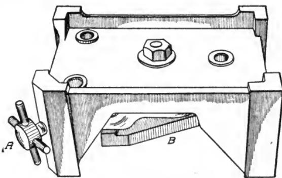
Fig. 375. Typical Open Box Drill Jig
