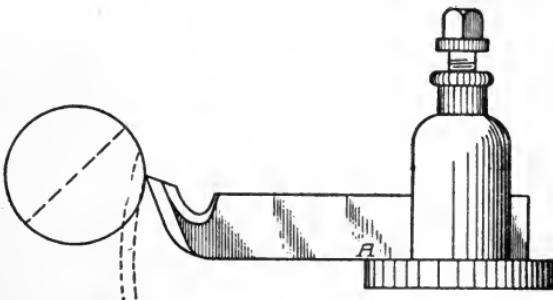
Fig. 185. Lathe Tool Improperly Set Up
