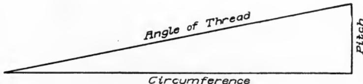
Fig. 274. Diagram for Finding Angle of Worm Thread
