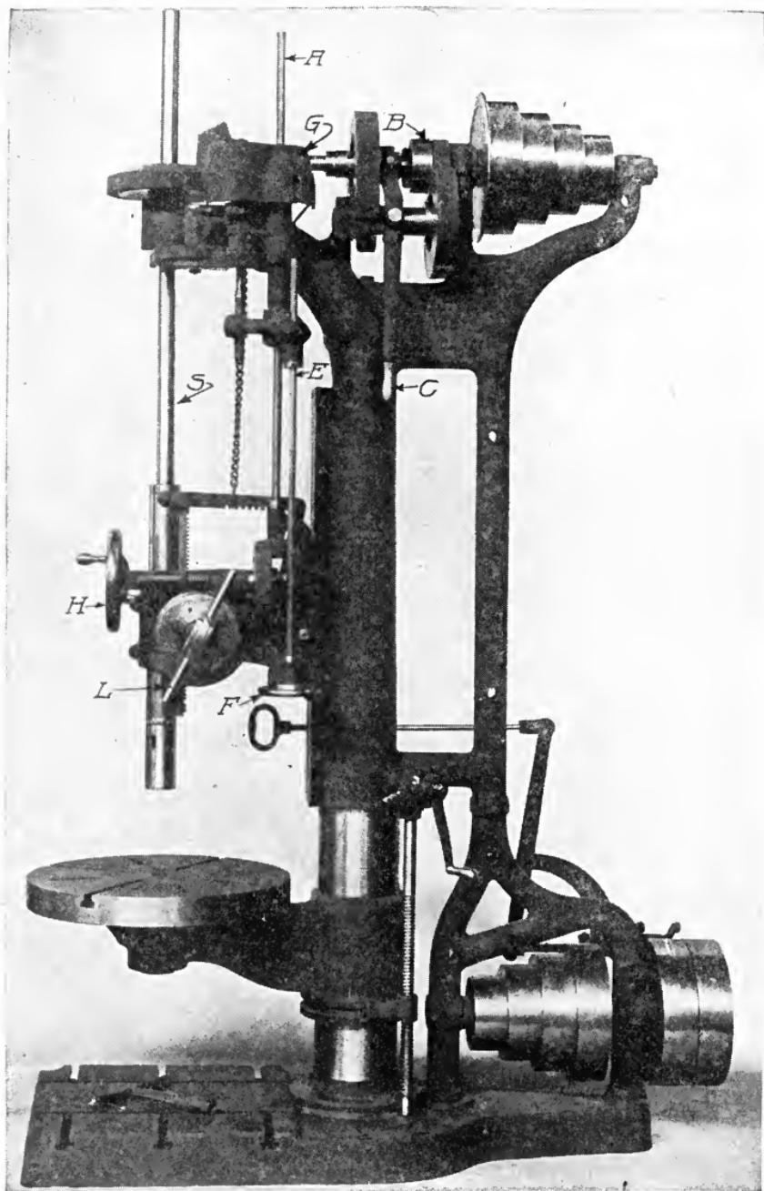
Fig. 175. Standard Power Feed Driller
