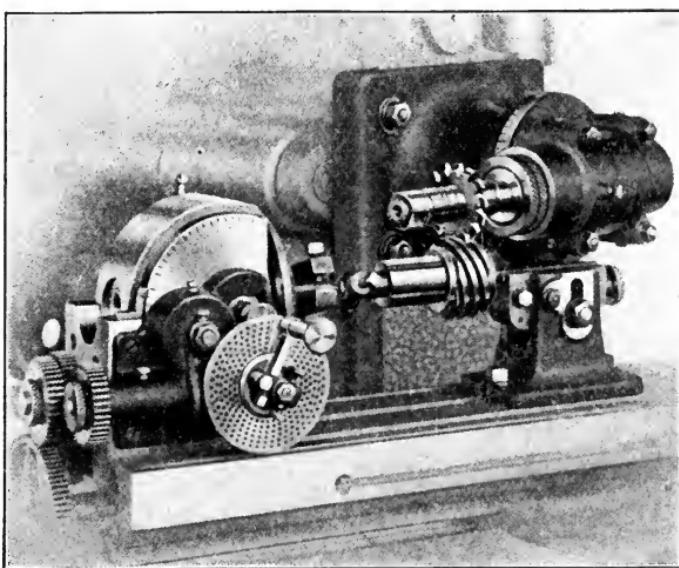
Fig. 239. Cutting Spiral with Milling Machine
