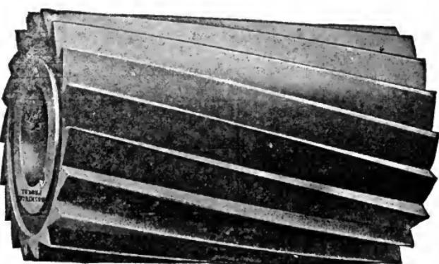
Fig. 201. Milling Cutter with Spiral Teeth
