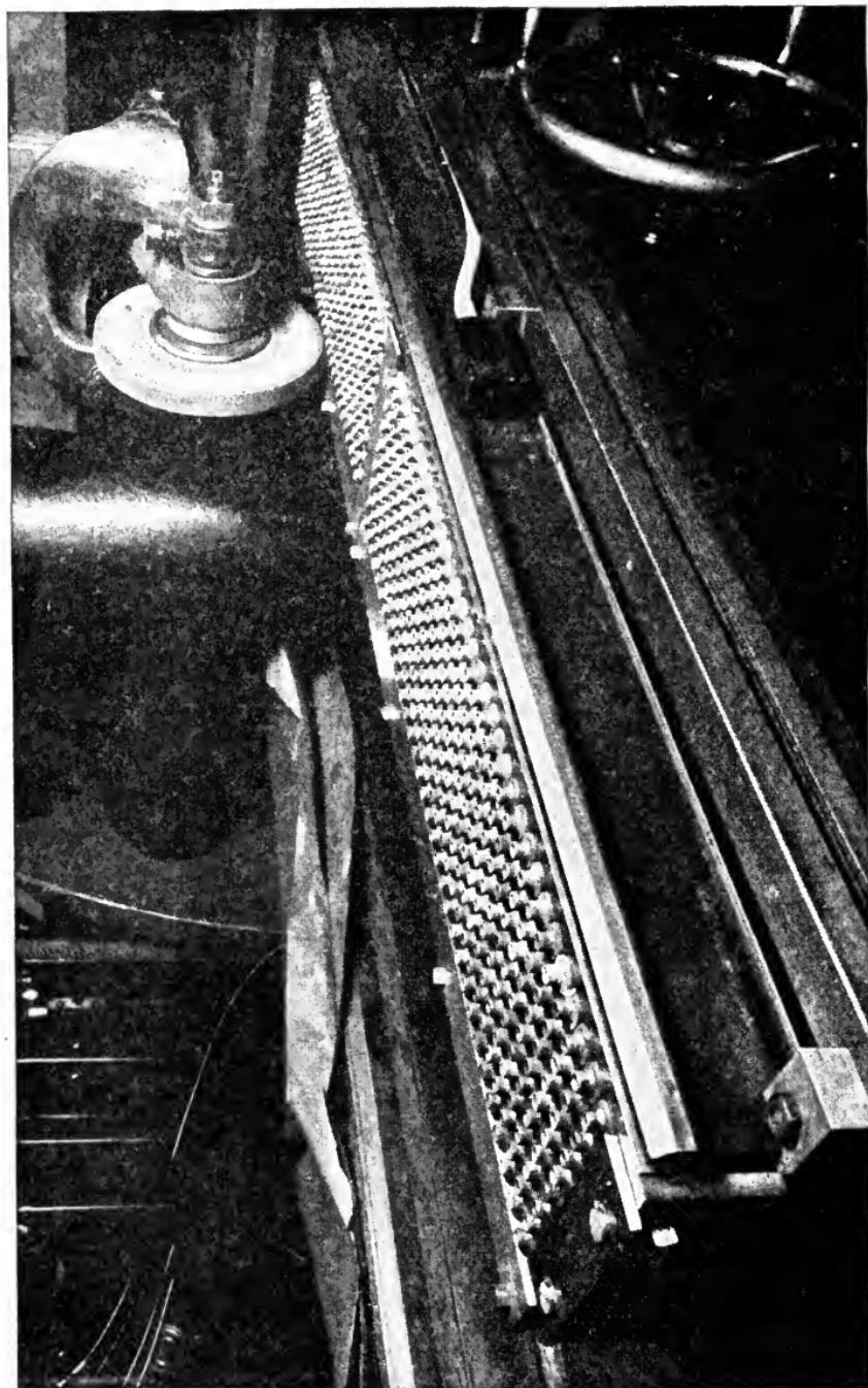
Fig. 397. Heald Magnetic Chucks Holding 528 Cones in Place for Grinding. With Ordinary Methods of Holding Work, Time Required 5 Hours; with Magnetic Chucks, Job Done in 1  $\frac{1}{2}$  Hours
