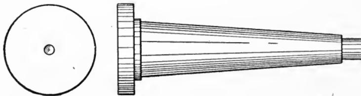
Fig. 170. Drill Pad for Flat Work
