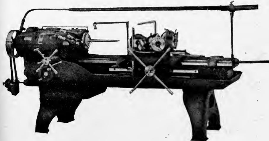
Fig. 299. Flat Turret Lathe, with Special Tools Bolted to Top of Flat Plate
