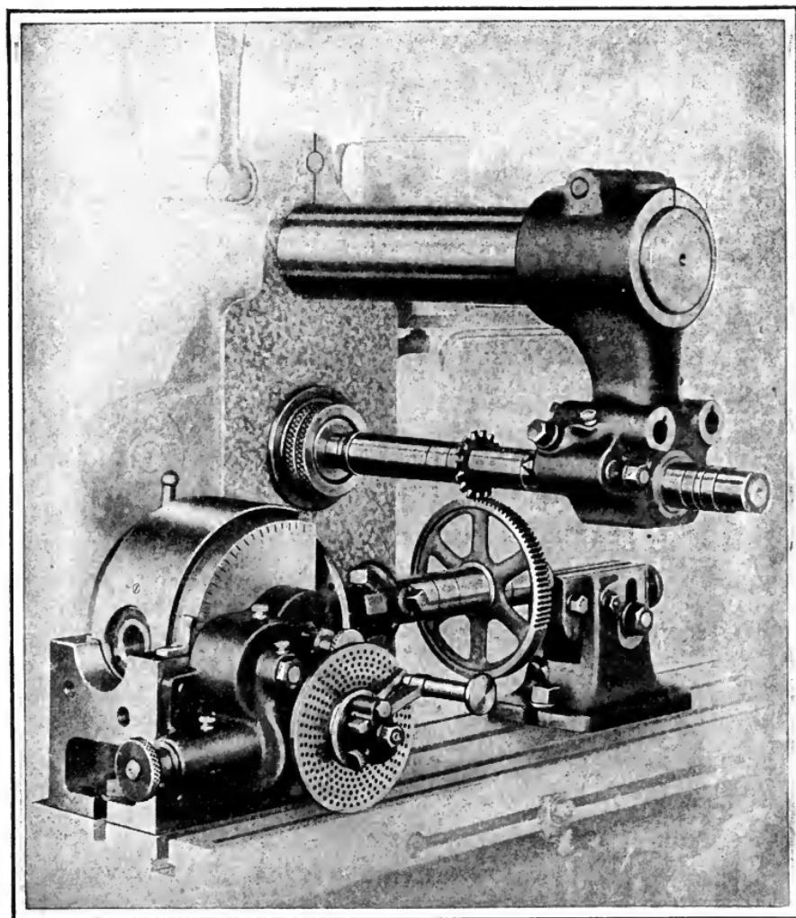
Fig. 242. Cutting Spur Gear on Milling Machine
