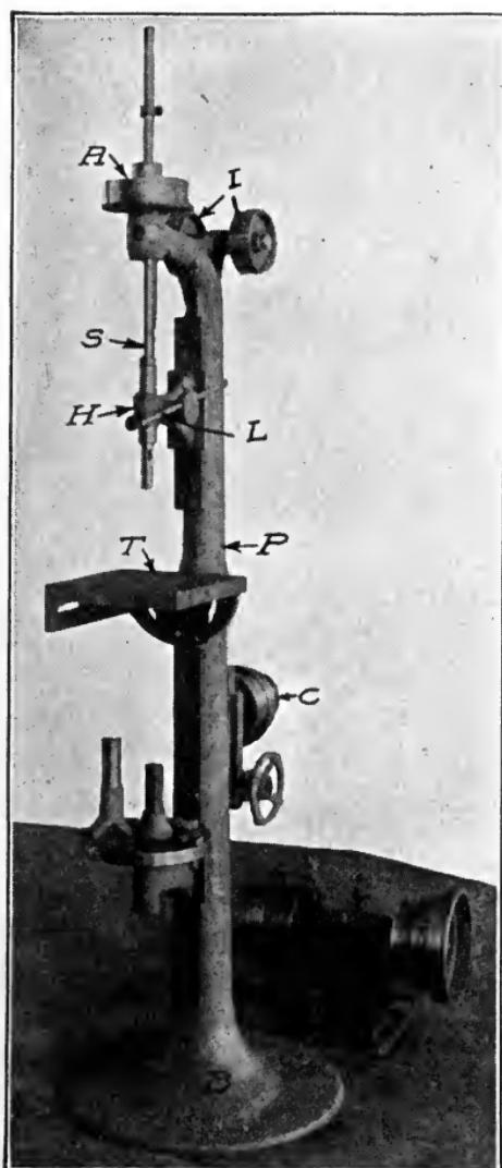
Fig. 174. Sensitive Driller
