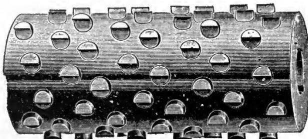
Fig. 212. Form of Inserted-Tooth Cutter Called Slabbing Cutter
