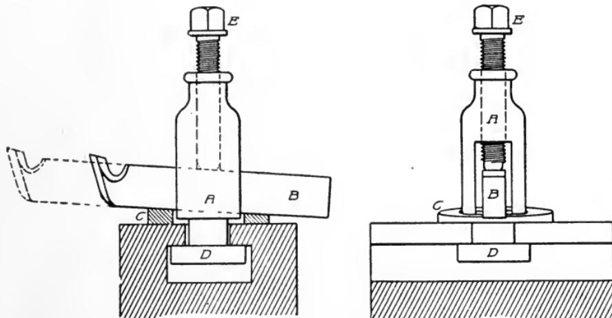
Fig. 118. Tool-Post Holding Tool to Carriage
