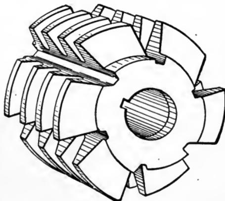
Fig. 278. Hob for Forming Teeth of Worm Gears
