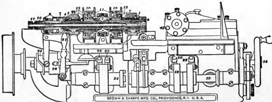
Fig. 319. Front Elevation of Brown and Sharpe Automatic Screw Machine, Showing Section through Spindle
