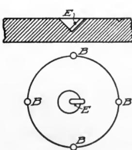
Fig. 179. Chiseling Countersink when not Concentric
