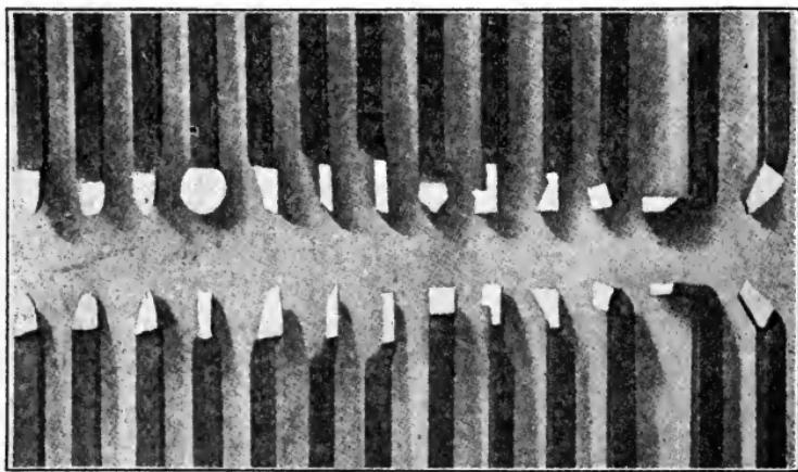
Fig. 371. Set of Planer Tools Ground on Sellers' Tool-Grinding Machine
