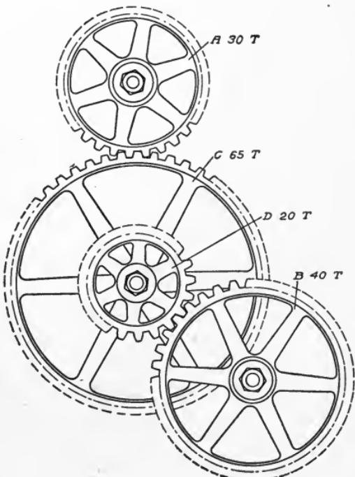
Fig. 166. Change-Gear Set-Up
