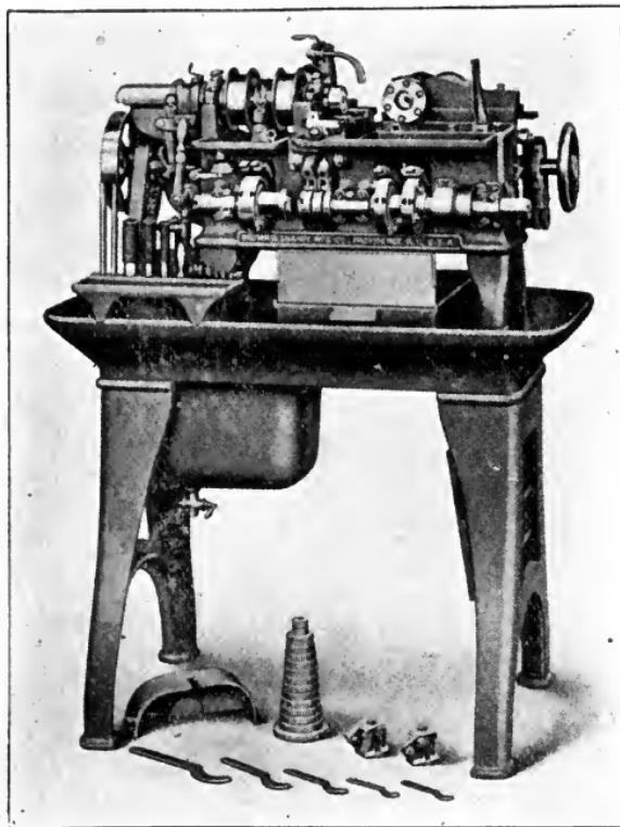
**Fig. 318.** Brown and Sharpe Automatic Screw Machine,
