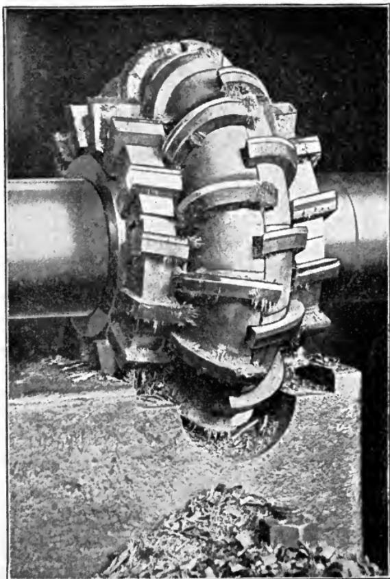
Fig. 346. Production Milling Cutter in Heavy Work
