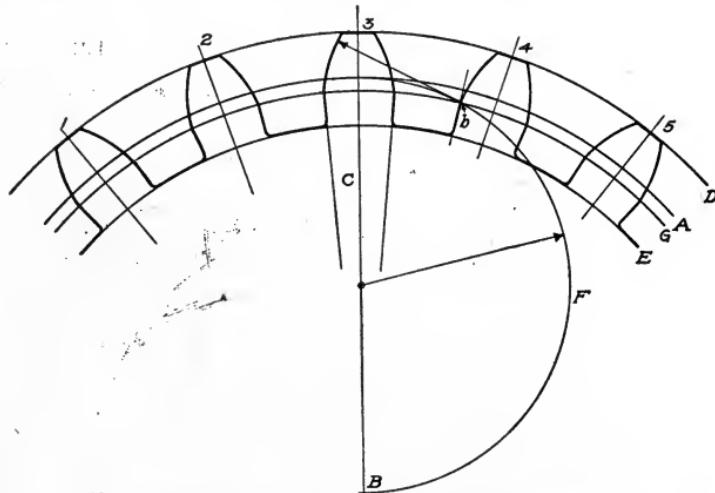
Fig. 265. Laying Out Gears of Second Class
