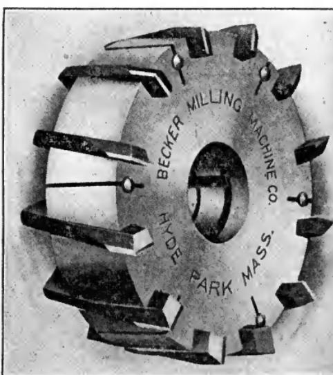
Fig. 218. End Mill with Inserted Teeth
