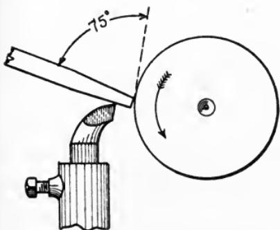
Fig. 89. Hand Tool Rest with Tool in Position
