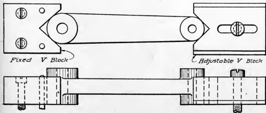
Fig. 379. Diagrams Showing Fixed and Adjustable V's
