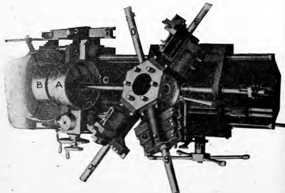
Fig. 312. Arrangement for Machining Inside of Cone Pulley
