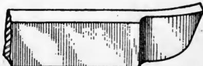
Fig. 127. Cutting-Off or Parting Tool
