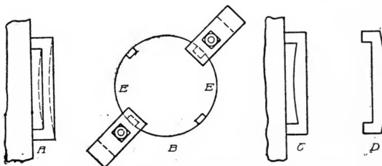
Fig. 136. Proper and Improper Method of Clamping Work
