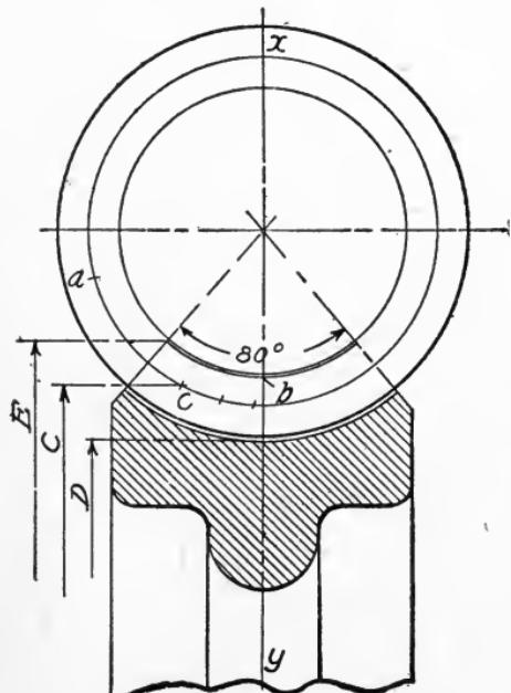
Fig. 273. Worm Gear with Large Enclosing Angle
