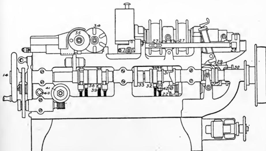
Fig. 320. Rear Elevation of Brown and Sharpe Automatic Screw Machine
