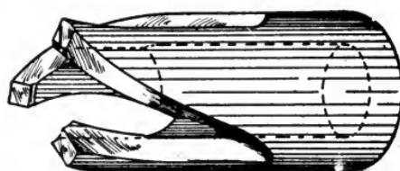
Fig. 322. Hollow Mill with Three Cutting Edges
