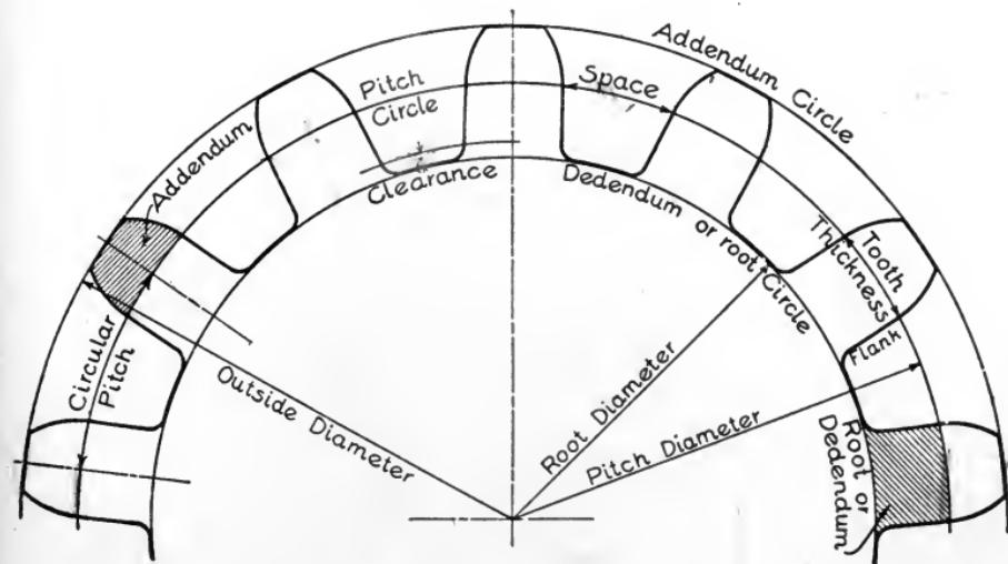
Fig. 261. Names of Tooth Parts
