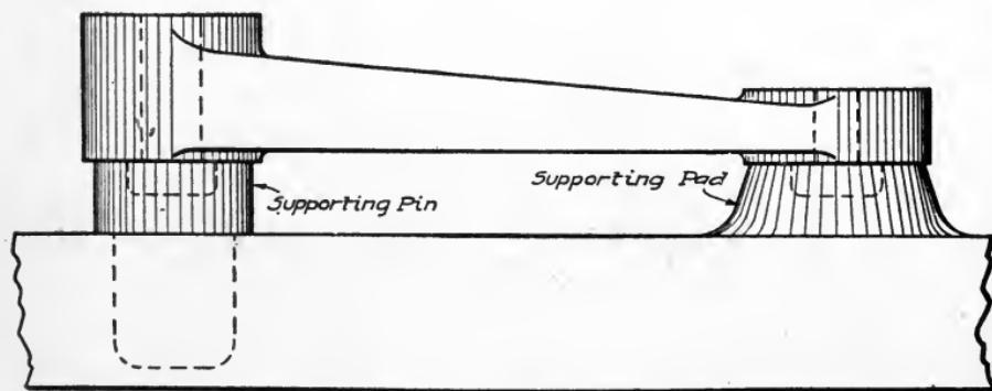
Fig. 381. Sketch Showing Adjustable Locating Points
