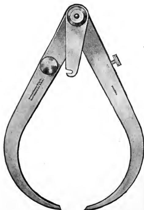
Fig. 17. Brown and Sharpe Outside Transfer Calipers
