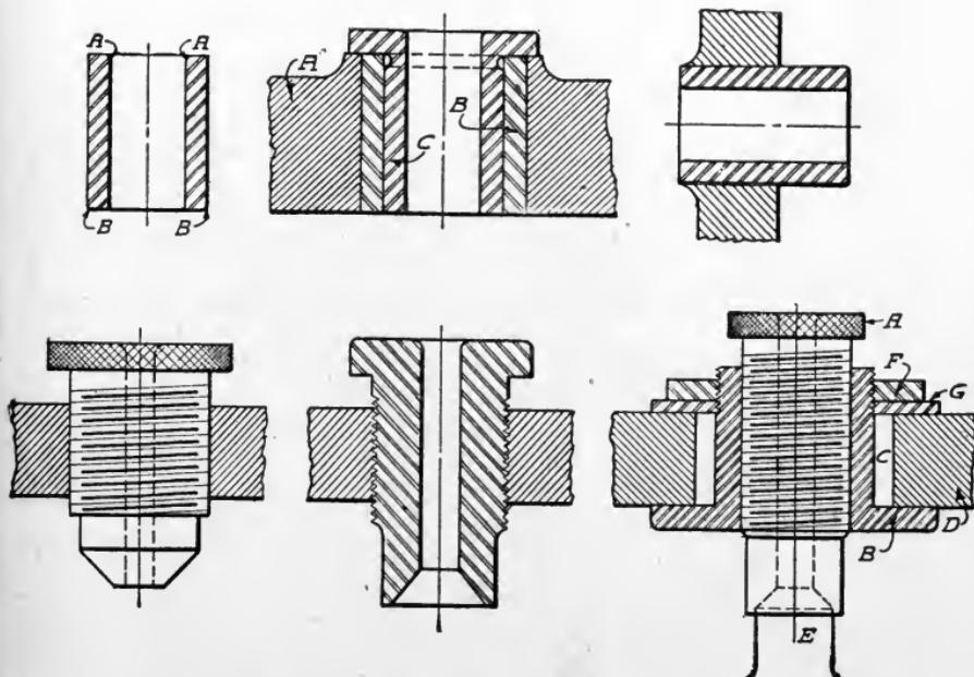
Fig. 384. Typical Bushings: Upper Line—Guiding Lining Bushings for Drill Jigs; Lower Left—Screw Bushing for Locating Work Central with Hole; Lower Center—Screw Bushing for Locating Round Work by Recesses; Lower Right—Floating Bushing
