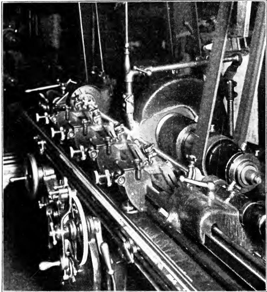
Fig. 325. Example of Steady Rests as Employed by Norton Grinding Company
