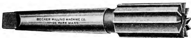
Fig. 215. Ordinary Form of End Mill
