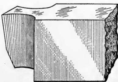
Fig. 158. Side View of Tool for Cutting Square Threads
