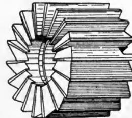
Fig. 220. Shell End Mill and Taper Shank for Holding It
