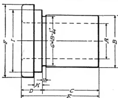
*Guide Bushings.* The soft body of the jig cannot be used to guide the drill if much service is required of the jig. In all production work, the guide holes for the drills are lined with hardened
