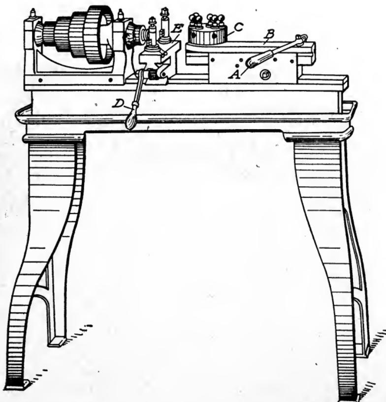
Fig. 292. Form of Monitor Lathe
