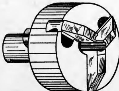
Fig. 324. Hollow Mill with Three Adjustable Blades
