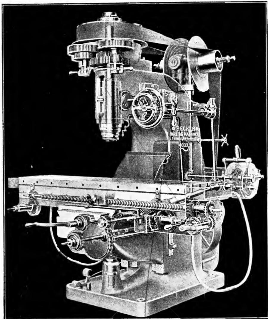
Fig. 230. Vertical Milling Machine with Working Parts Shown in Ghost
