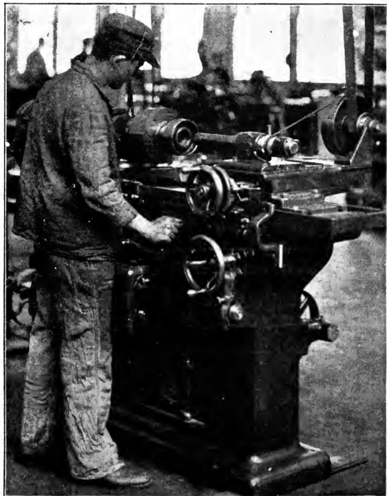
Fig. 398. Heald Internal Grinder Fitted with Magnetic Chuck
