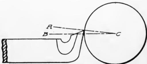
Fig. 117. Standard Setting with Cutting Edge of Tool a Little Above Center
