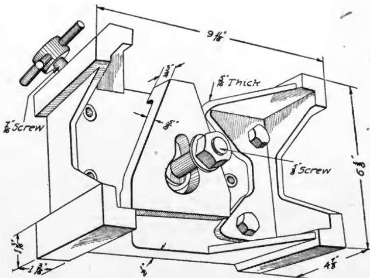
Fig. 376. Bottom View of Box Drill Jig Shown in Fig. 375
