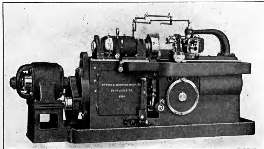
Fig. 314. Latest Type of Automatic Chucking and Turning Machine
