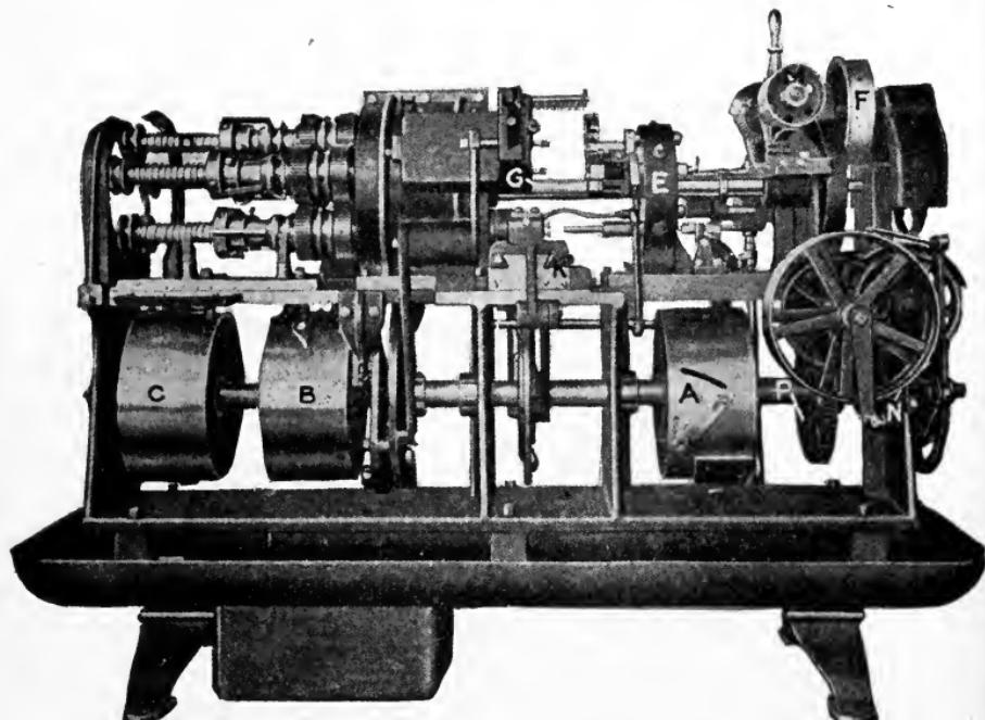
Fig. 317. Universal Multiple-Spindle Automatic Screw Machine
