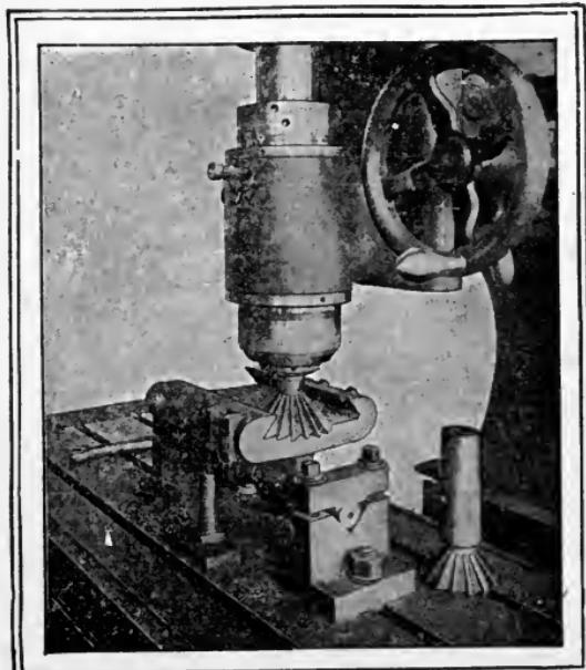
Fig. 236. Dovetail Cutter on Vertical Milling Machine
