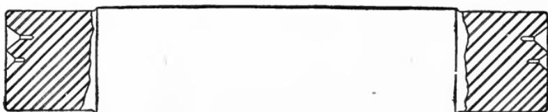
Fig. 150. Mandrel for Holding an Eccentric
