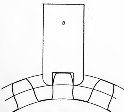
Fig. 282. Sheet-Metal Gage for Measuring Width of Teeth
