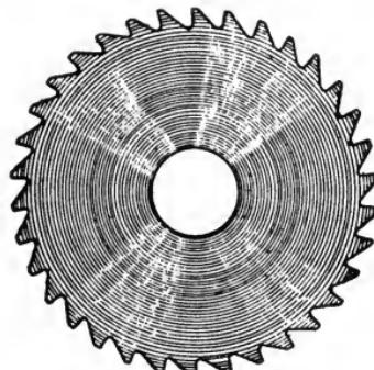
Fig. 204. Slitting Saw
