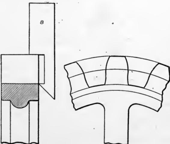
Fig. 281. Sheet-Metal Gage for Measuring Depth of Teeth
