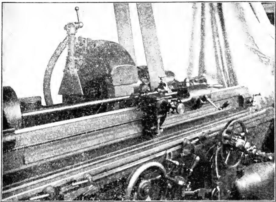
Fig. 329. Norton Grinder with 5 $\frac{1}{4}$ -Inch Face Wheel for Grinding Ford Axles and Drive Shafts
