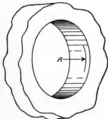
Fig. 138. Centering a Hollow Piece
