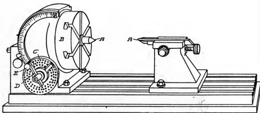
Fig. 243. Gear Cutter with Divided Head
