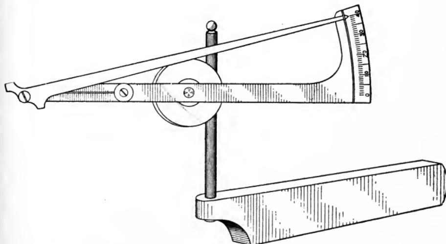
Fig. 140. Starrett Indicator Used for Centering Work
