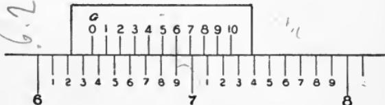
Fig. 32. Position of Vernier for Example 6
