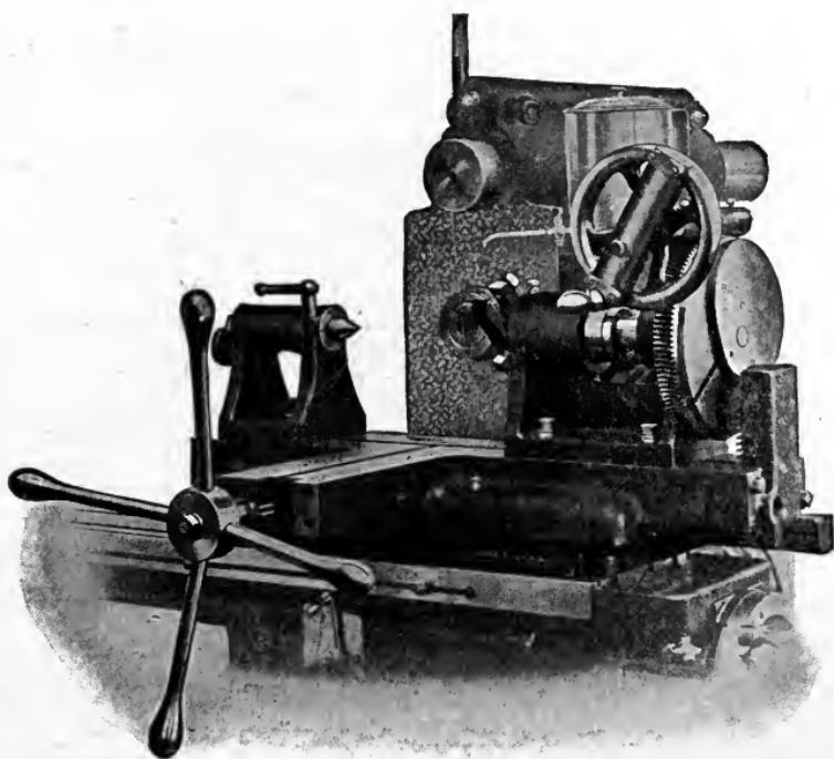
Fig. 241. Cam-Cutting Attachment for Milling Machine
