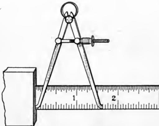
Fig. 18. Setting Inside Calipers
