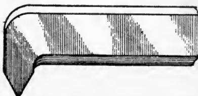
Fig. 161. Internal Threading Tool
