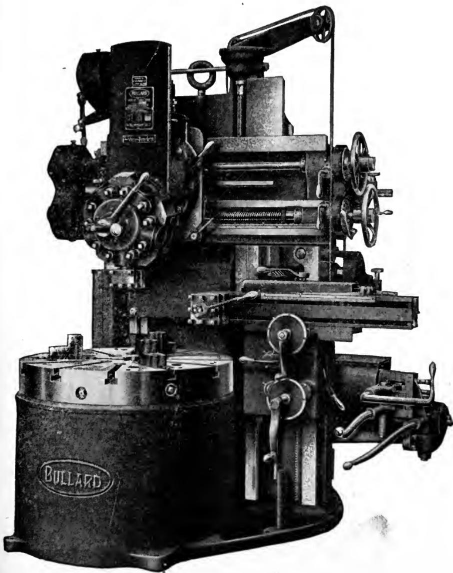
Fig. 353. Bullard Vertical Turret Lathe
