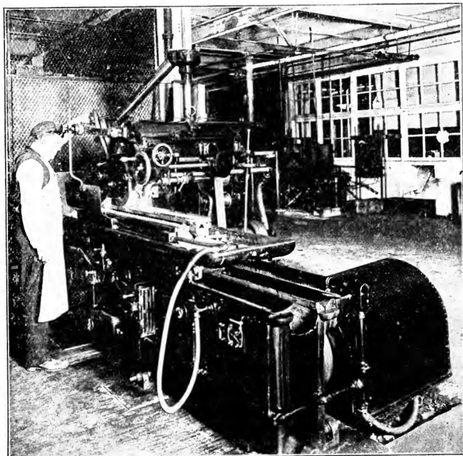
Fig. 338. Example of Flat Surface Grinding
