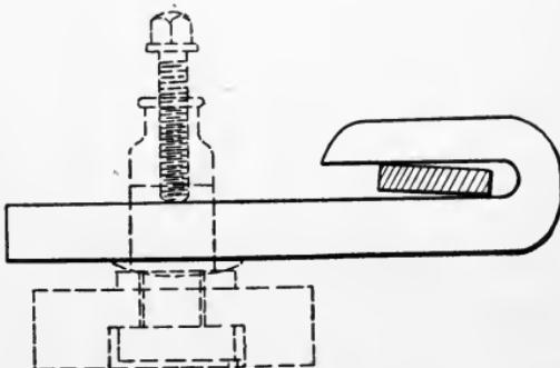
Fig. 64. Chucking Drill Rest
