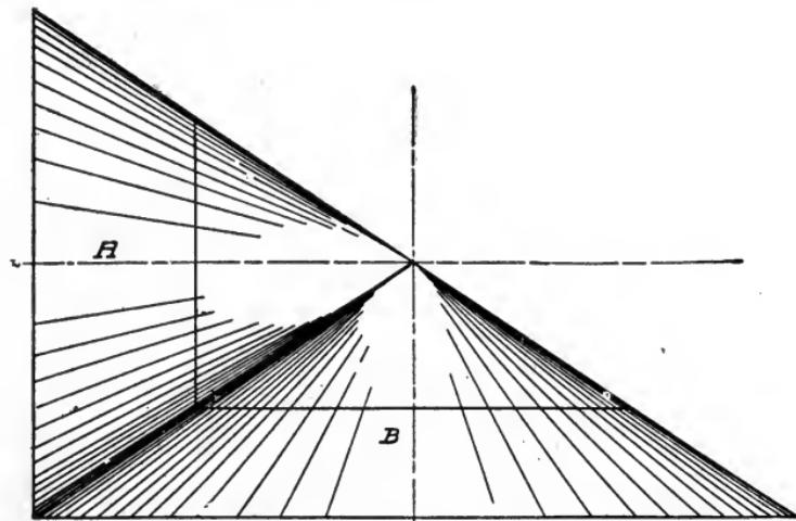
Fig. 259. Two Cones in Contact
