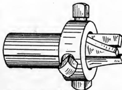
Fig. 323. Improved Hollow Mill
