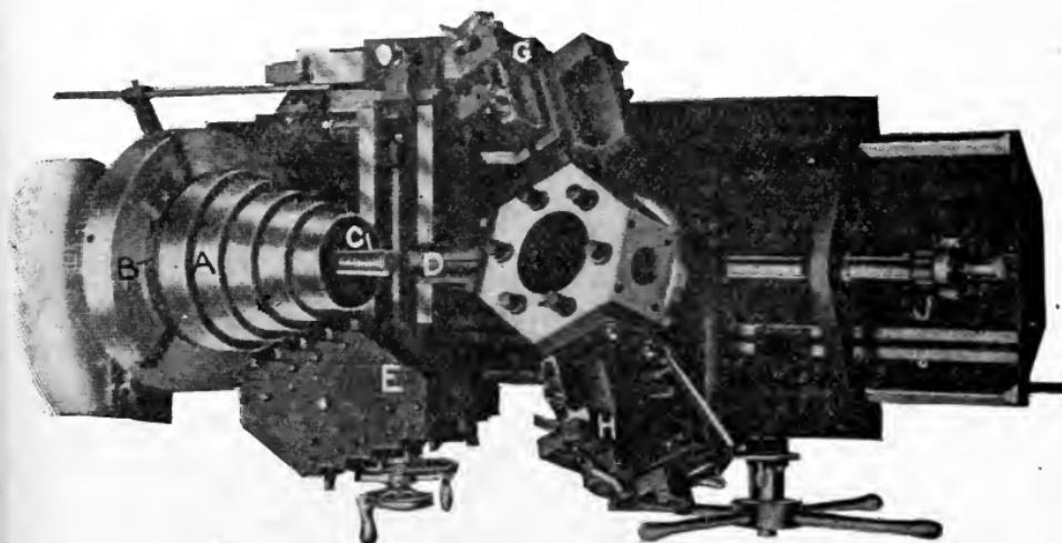
Fig. 311. Turret Lathe Arranged to Machine Outside of Cone Pulley
