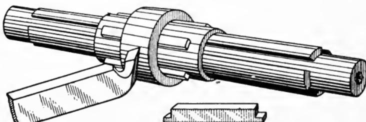
Fig. 112. Diagram Showing Use of Expanding Mandrel
