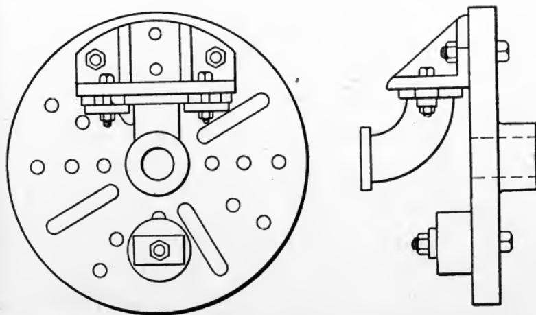
Fig. 137. Angle Iron Clamped to Faceplate and Counterbalanced
