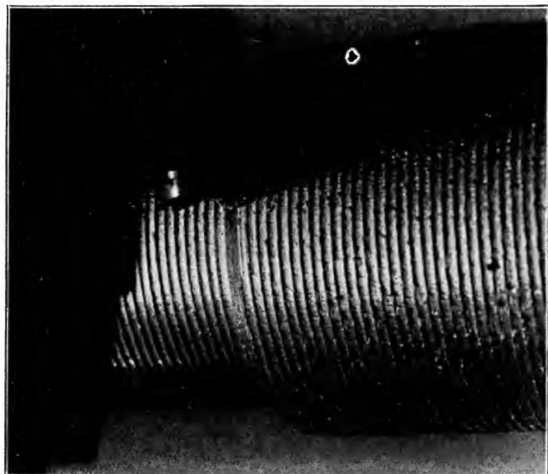
Fig. 327. Roughing-Out for Grinding Showing Heavy Cut
