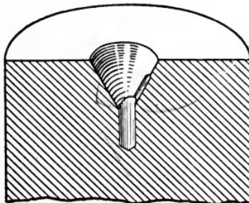
Fig. 143. Method of Drawing the Hole
