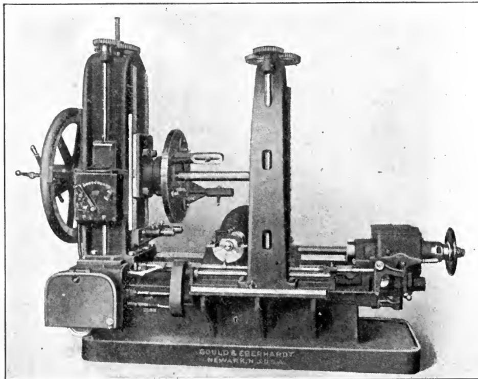
Fig. 285. "New Type" Gear-Cutting Machine Entirely Automatic for Cutting Spur Gears Only
