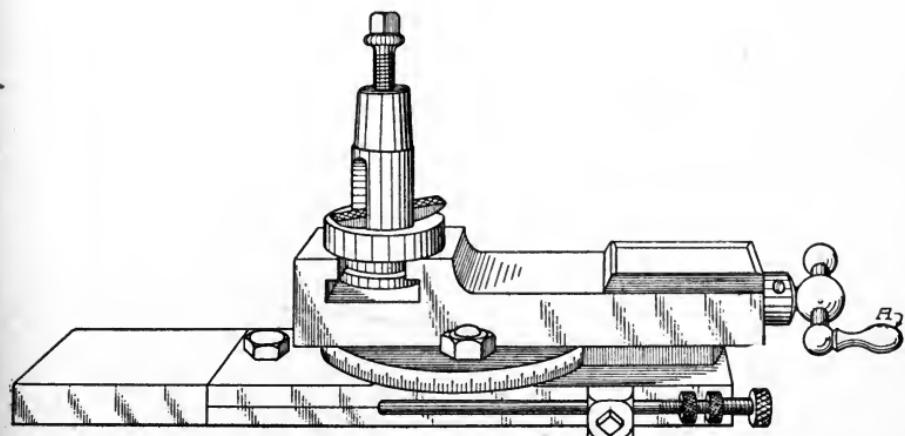
Fig. 146. Compound Tool Slide
