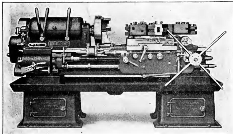
Fig. 298. "Prentice" High-Speed Turret Lathe
