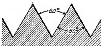
Fig. 155. Section of V-Thread
