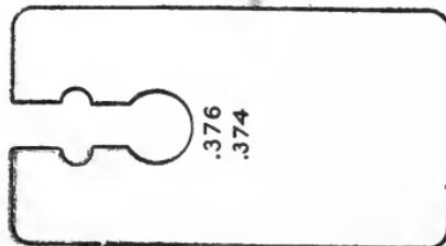
Fig. 38. Limit Gage with Jaws in Series
