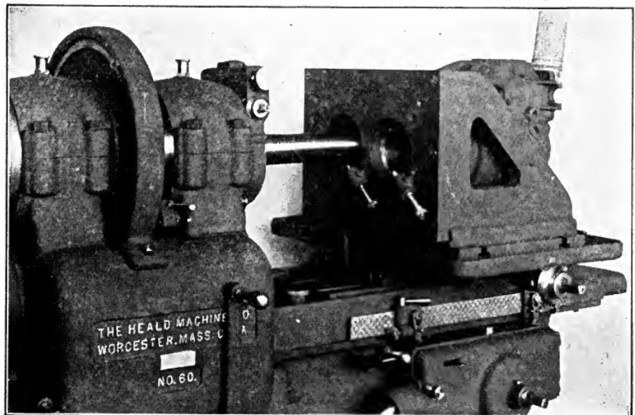
Fig. 335. Grinding Gas Engine Cylinders. Same Set-Up as Fig. 334, Showing Holding Jig and Turning Tool at Mouth of Hole
