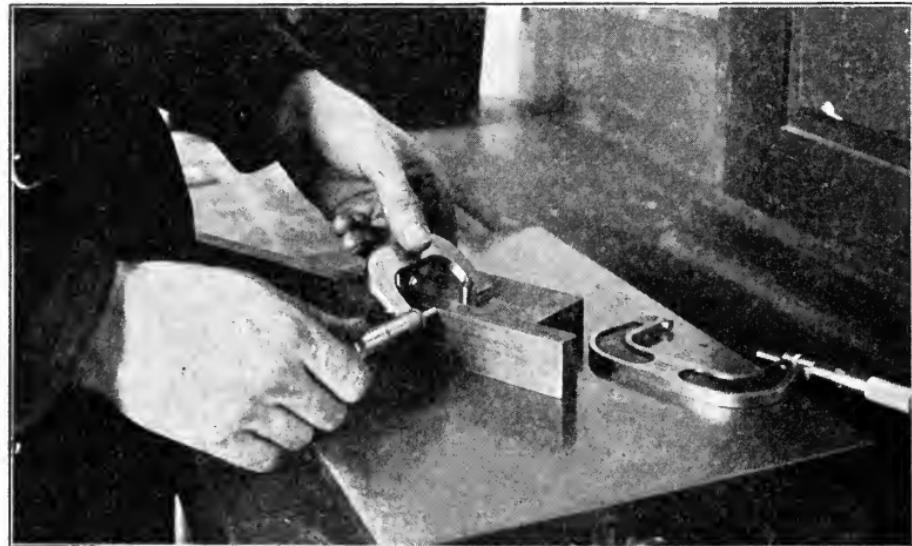
Fig. 386. Positioning Buttons with Micrometer Caliper
