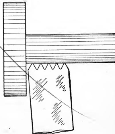
Fig. 167. Hand Chaser Cutting Outside Thread
