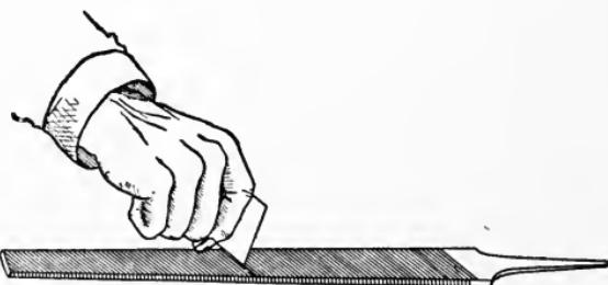
Fig. 55. Removing Pins from a File
