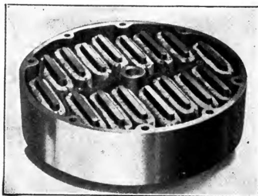
Fig. 400. View of Magnetic Chuck Casting
