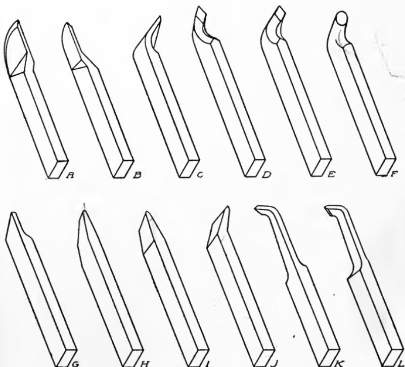
Fig. 131. Common Forms of Slide-Rest Tools. *A*—Left-Hand Side; *B*—Right-Hand Side; *C*—Right-Hand Bent; *D*—Right-Hand Diamond Point; *E*—Left-Hand Diamond Point; *F*—Round Nose; *G*—Cutting-Off; *H*—Roughing; *I*—Threading; *J*—Bent Threading; *K*—Boring; *L*—Inside Threading
