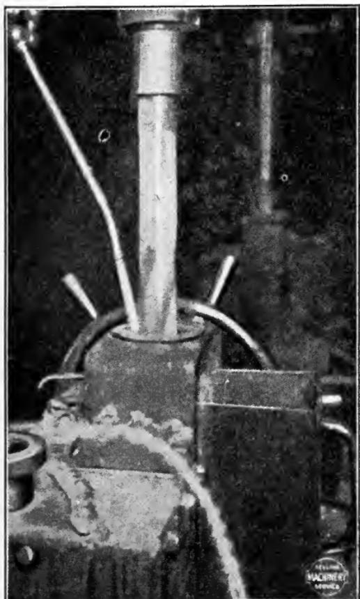
Fig. 374. Drilling Operation Showing How Lubricant Floods the Work
