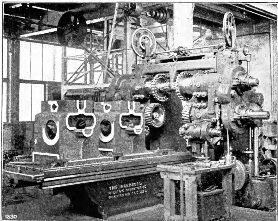
Fig. 343. Ingersoll Horizontal Milling Machine, Milling Gasoline Traction Engine Frames.  $\frac{1}{2}$  Inch of Metal Removed from each of Six Surfaces. 14 Bases Finished in 10 Hours.
