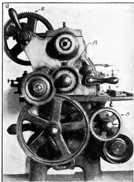
Fig. 165. Compound Lathe Gearing
