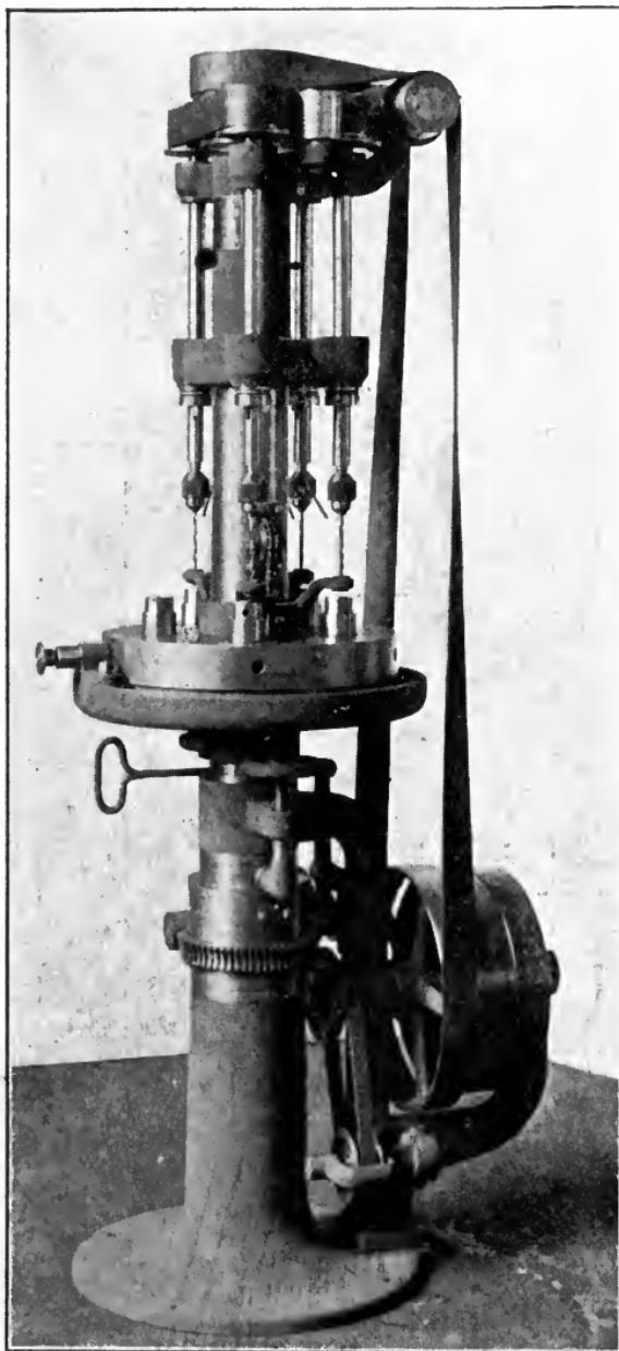
Fig. 350. "Single Purpose" Bemis Driller
