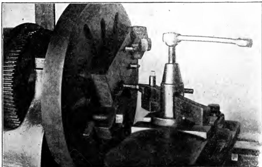
Fig. 388. Boring Hole for Guide Bushing
