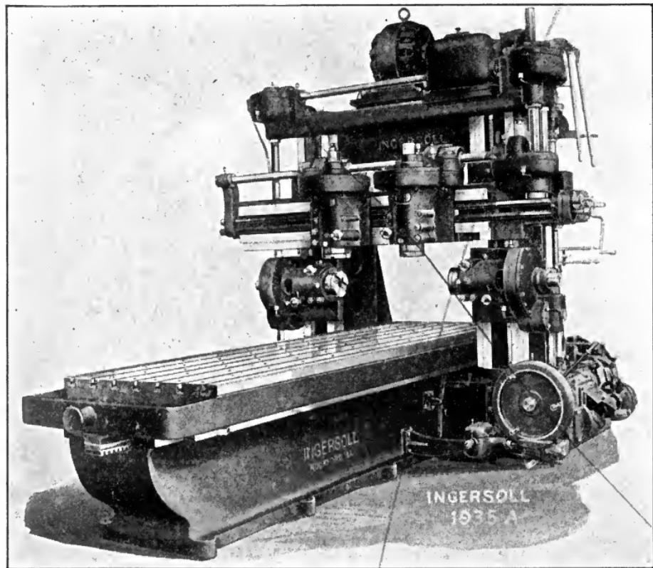
Fig. 226. Planer Type Four-Spindle Milling Machine
