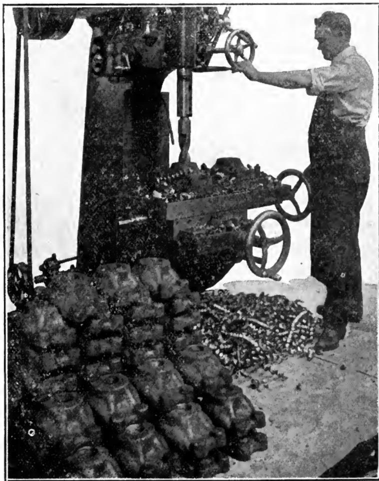
Fig. 348. Baker Driller Driving 2½-Inch Drill through Drop-Forged Wrought-Iron Saddles
