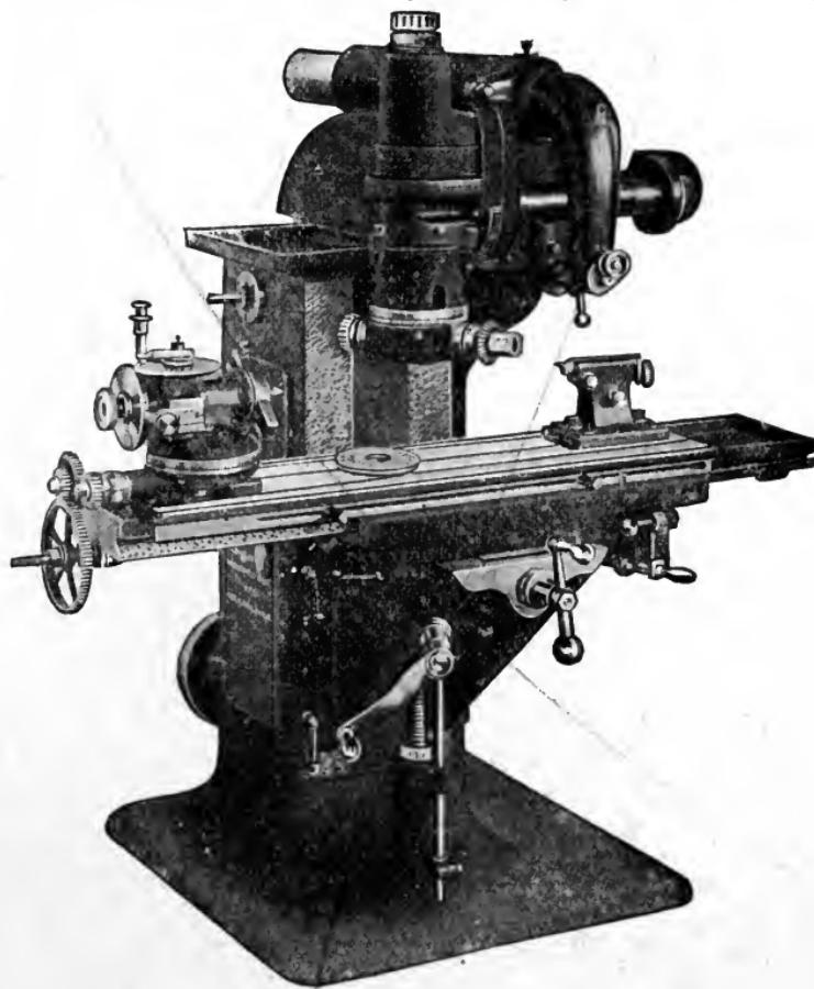
Fig. 231. Duplex Milling Machine Set for Cutting Spirals
