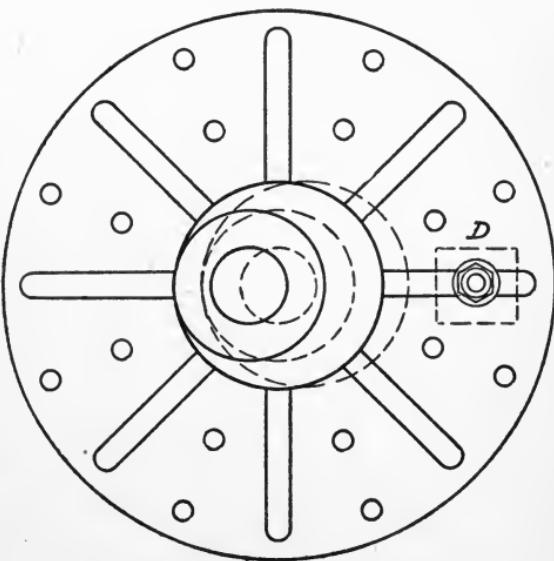
Fig. 151. Piece Mounted on Faceplate for Eccentric Turning
