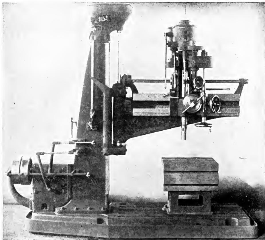
Fig. 177. Radial Driller with Four-Foot Arm for Heavy Duty
