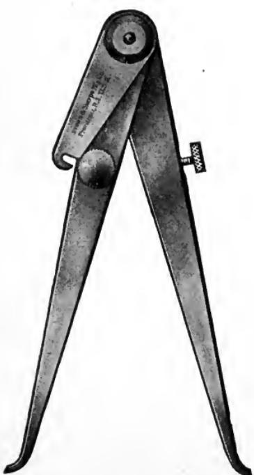
Fig. 16. Brown and Sharpe Inside Transfer Calipers
