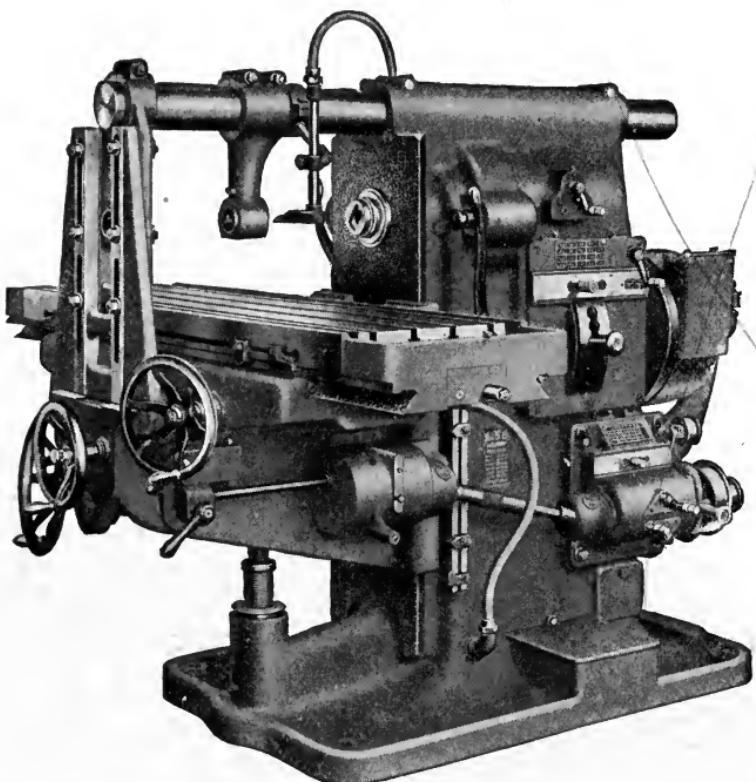
Fig. 224. Horizontal Milling Machine—Column Type
