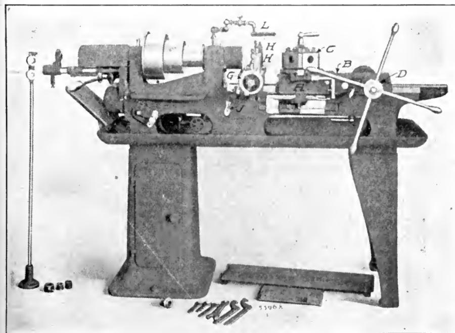
Fig. 295. Turret Lathe, Hand-Revolved and Hand-Fed
