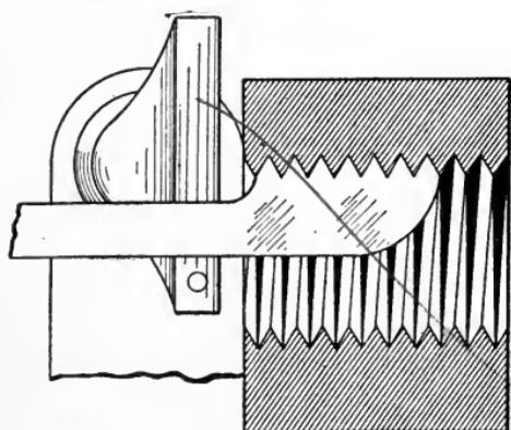
Fig. 168. Hand Chaser Cutting Inside Thread
