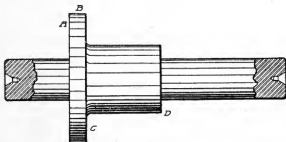
Fig. 145. Turning Taper on Piece Held by Mandrel
