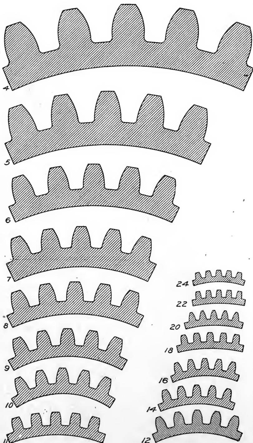
Fig. 262. Proportions of Teeth of Different Diametral Pitches
