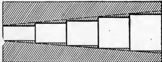
Fig. 80. Method of Stepping Holes before Using Taper Reamer
