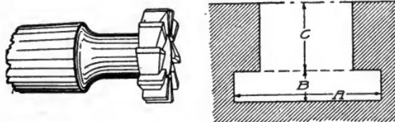
Fig. 216. T-Slot Milling Cutter and Section of Slot
