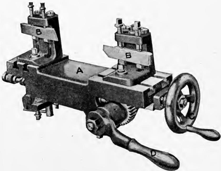
Fig. 308. Cross-Slide Carrying Two Tools
