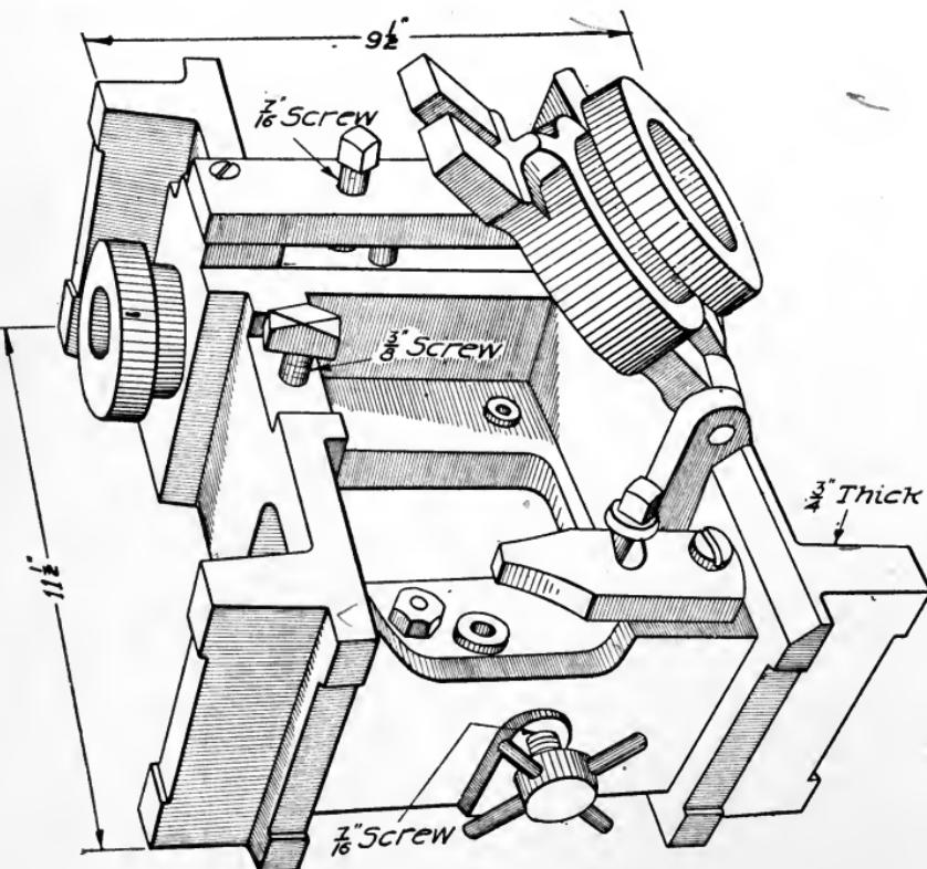
Fig. 377. Two Views of Closed Box Drill Jig
