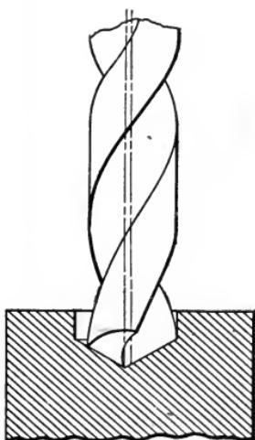
Fig. 69. Drill with Lips of Unequal Length
