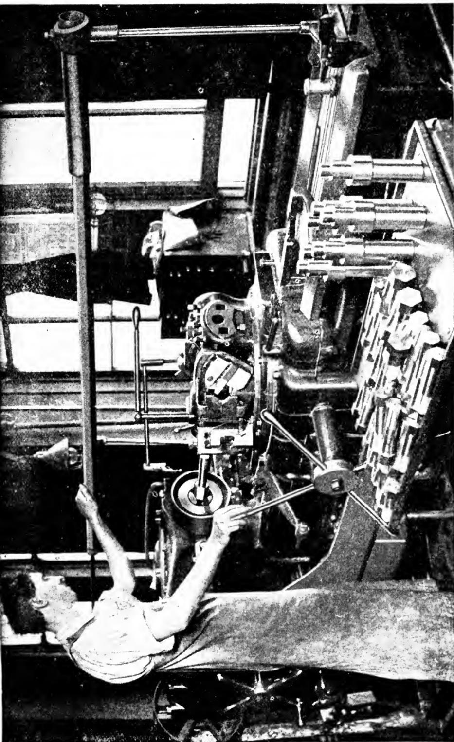
Fig. 355b. Jones and Lamson "Hartness" Turret Lathe Finishing Bar Work. Time 45 Minutes per Piece
