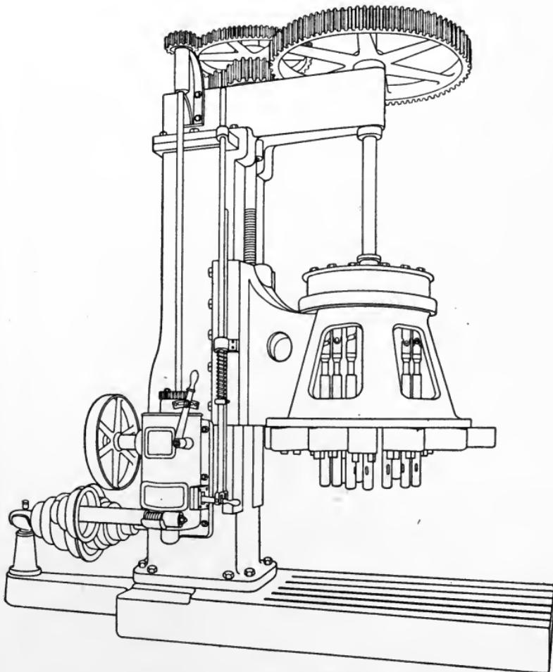
Fig. 176. Typical Multi-Spindle Driller
