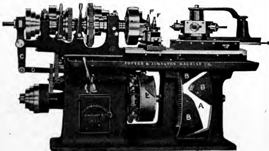
Fig. 313. Automatic Chucking and Turning Machine
