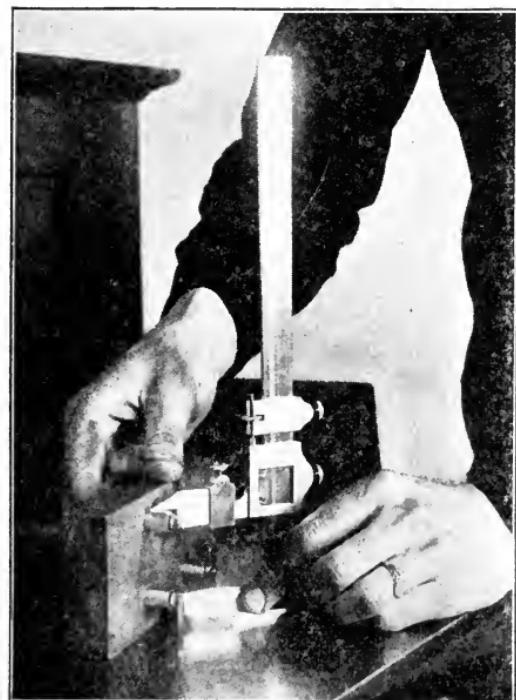
Fig. 387. Positioning Buttons with Vernier Caliper
