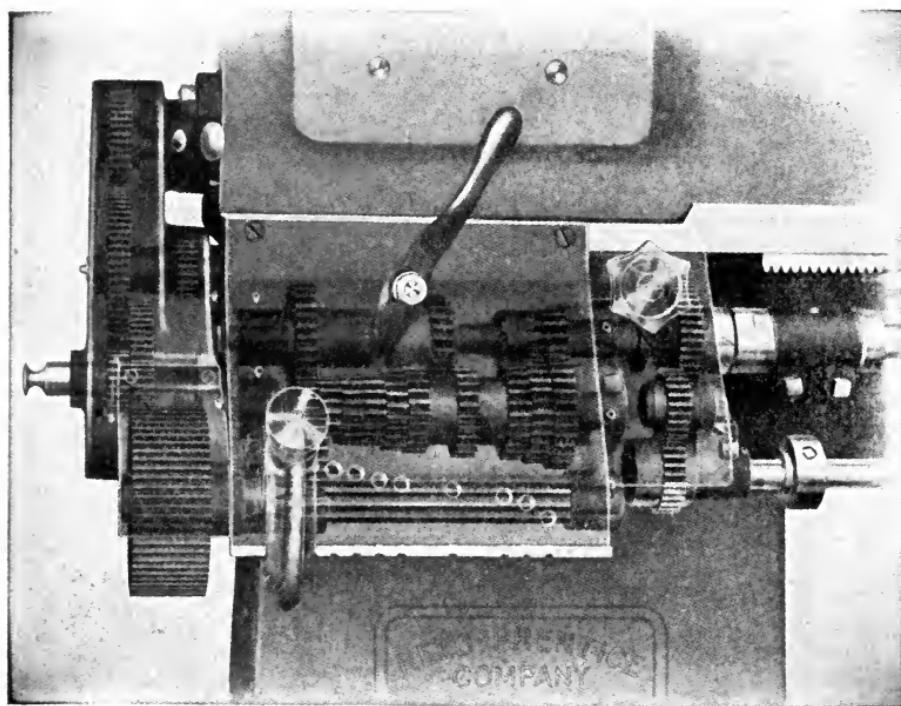
Fig. 352. Transparent View of "Reed" Quick-Change Gear Mechanism
