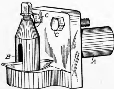
Fig. 306. Turret Holder for Tool-Post
