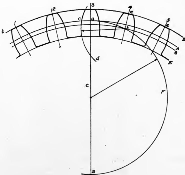
Fig. 264. Laying Out Large Gears
