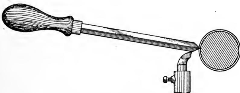
Fig. 92. Position of Tool for Turning Steel
