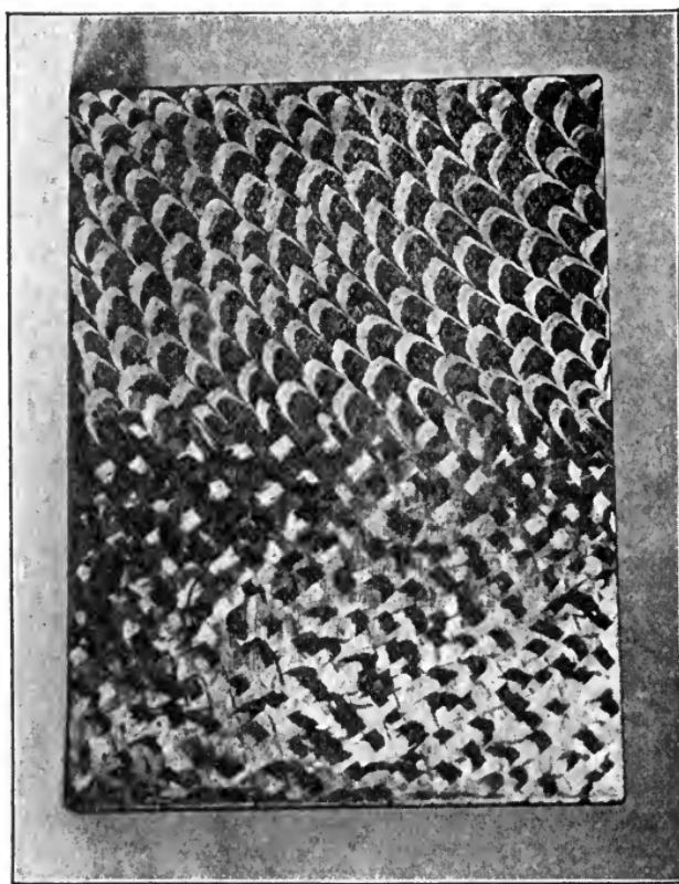
Fig. 389. Typical "Spotting" Pattern on Surface Plate
