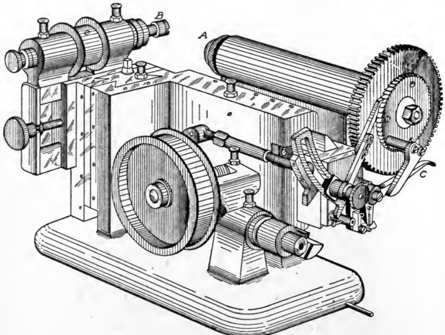
Fig. 287. Bench Gear Cutter
