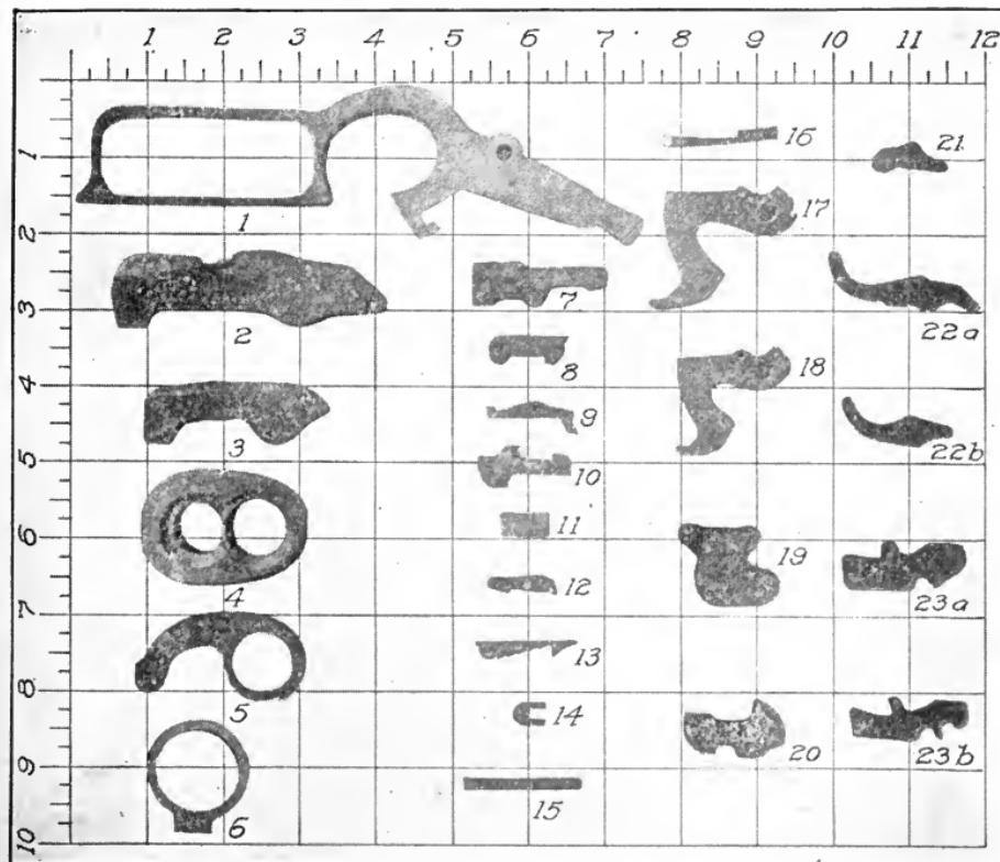
Fig. 340. Gun Parts Ground on Vertical Grinder
