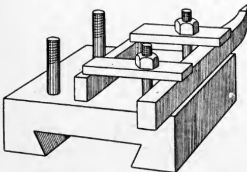
Fig. 119. Tool Holder for Heavy Turning
