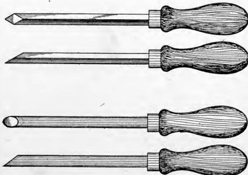
Fig. 91. Typical Hand Tools for Steel Turning
