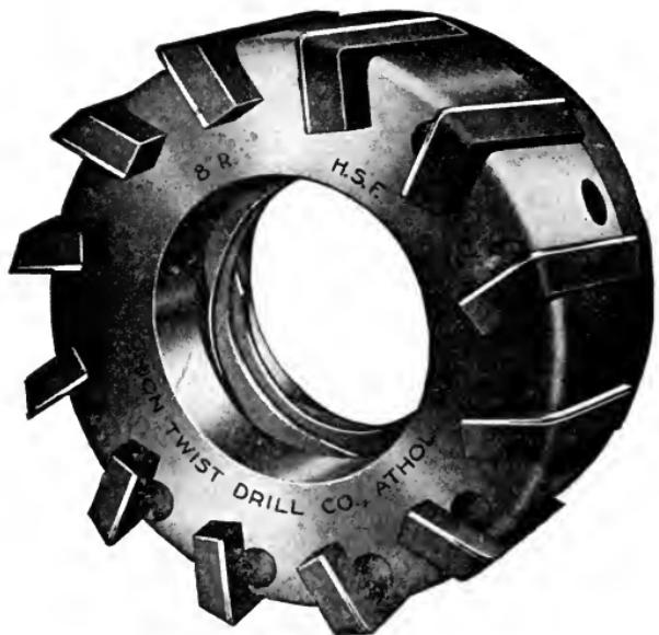
Fig. 345. High-Power Face Mill with High-Speed Steel Teeth
