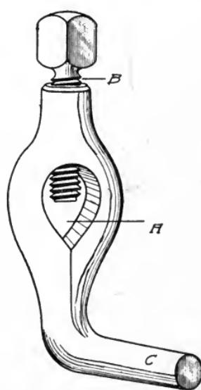
Fig. 107. Lathe Dog for Round Work
