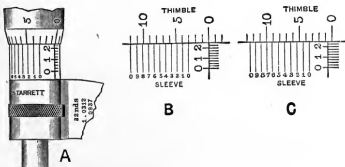
Fig. 23. Diagrams Showing How to Read Micrometer Caliper
