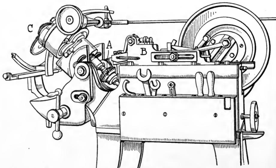
Fig. 290. Gear-Planing Machine
