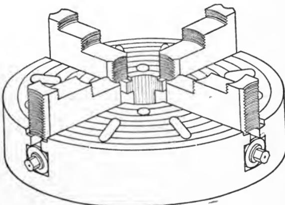
Fig. 104. Lathe Work Chuck
