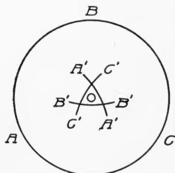
Fig. 250. Centering Round Bar to be Turned in Lathe
