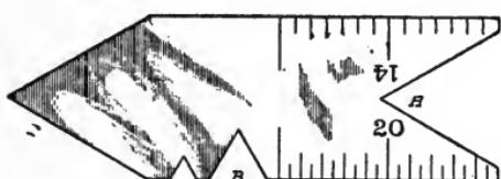
Fig. 162. Thread or Center Gage
