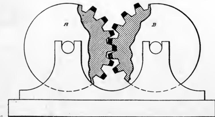
Fig. 260. Tooth Gears in Contact
