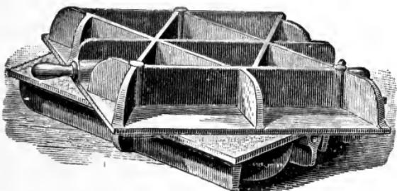
Fig. 41. Cast-Iron Surface Plate
