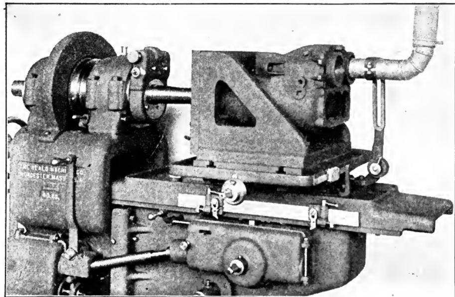
Fig. 334. Grinding Gas Engine Cylinders. View Shows Exhaust for Dust, Jig for Holding Cylinders, and Eccentric Wheel Spindle
