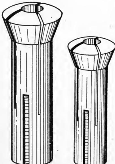
Fig. 221. Typical Spring Collets
