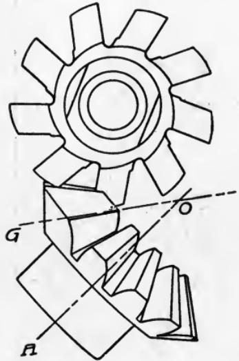
Fig. 244. Cutting a Bevel Gear
