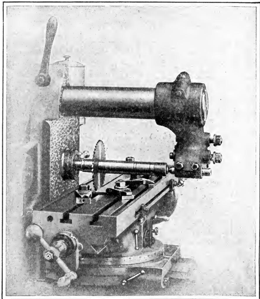
Fig. 198. Sawing Flat Stock
