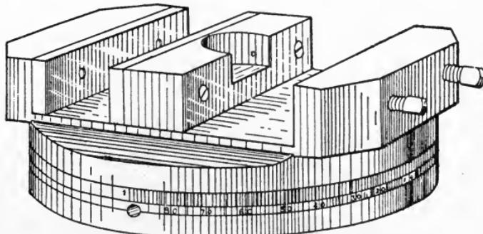
Fig. 189. Planer Chuck for Holding Work
